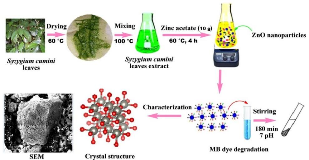
**Figure 7.** Preparation scheme of ZnO nanoparticles. Reprinted with permission from Ref. [37], Copyright 2021 Elsevier.
