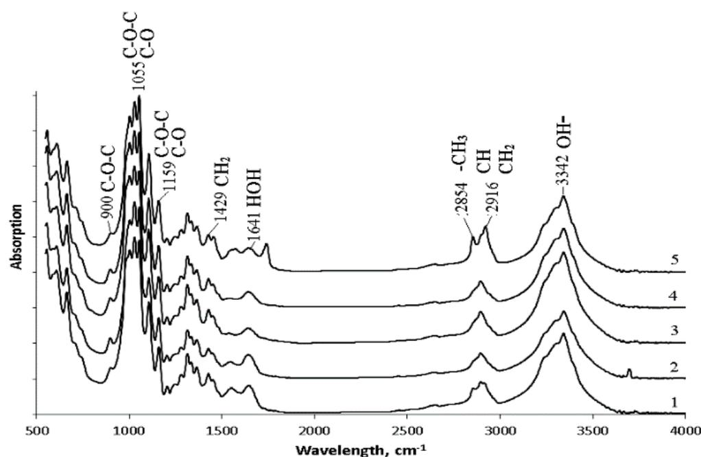
**Figure 6.** FTIR spectrum data of BC synthesized on various C-substrates: 1—glucose; 2—glucose + oil; 3—molasses; 4—glycerol; 5—sprat oil.
