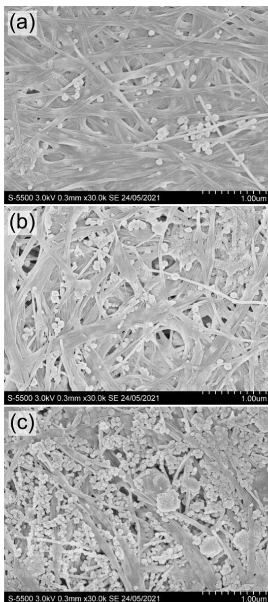
**Figure 8.** SEM images of BC/AgNP films with different Ag content in the composite: (a) 0.06; (b) 0.21; (c) 0.46 mg/cm<sup>2</sup> (obtained at a concentration of AgNO<sub>3</sub> in solution, respectively, 0.01; 0.05; 0.10 g/L). Bar = 1 µm.
