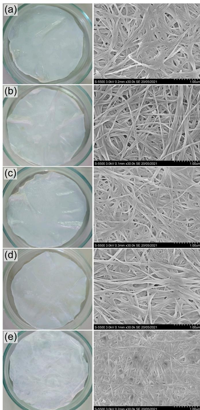
**Figure 5.** Photo and SEM images of BC films synthesized on various C-substrates: (a) glucose; (b) glucose + oil; (c) molasses; (d) glycerol; (e) sprat oil. Bar = 1 µm.
