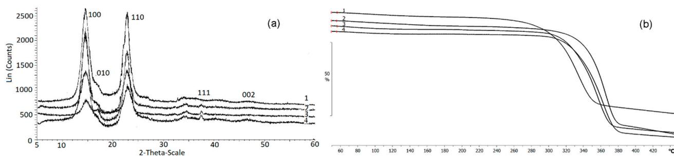
**Figure 9.** X-Ray (a) and TGA (b) data of BC and BC/AgNp composites: (1)—pristine BC; (2–4)—BC/AgNp composites obtained at different initial concentration of  $\text{AgNO}_3$  in solution, respectively, 0.01; 0.05; 0.10 g/L.
