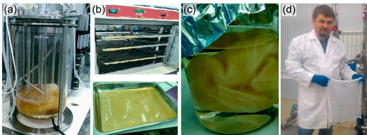
**Figure 4.** The two-stage process of BC production: (a) production of inoculum in submerged culture with stirring; (b) BC synthesis in surface liquid-phase mode; (c) cleaning of BC films from bacteria and medium components; (d) finished product.
