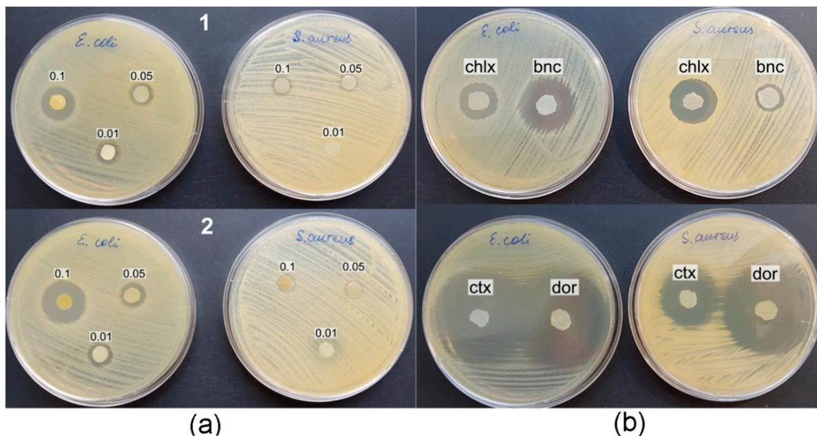
**Figure 10.** Antibacterial activity of BC composites against reference strains *E. coli* and *S. aureus*; (a) BC/AgNPs composites: 1—boiling BC in silver nitrate solution, 2—immersion of BC in silver nitrate solution for 9 days; (b) BC/antibiotic composites: *chlx*—BC/chlorhexidine, *bnc*—BC/baneocin, *ctx*—BC/cefotaxime, *dor*—BC/doripenem.
