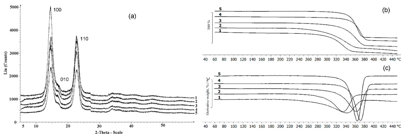
**Figure 7.** X-Ray (a) and TGA (b,c) data of the BC synthesized on various C-substrates; (b) beginning of destruction; (c) destruction rate; 1—glucose; 2—glucose + oil; 3—molasses; 4—glycerol; 5—sprat oil.
