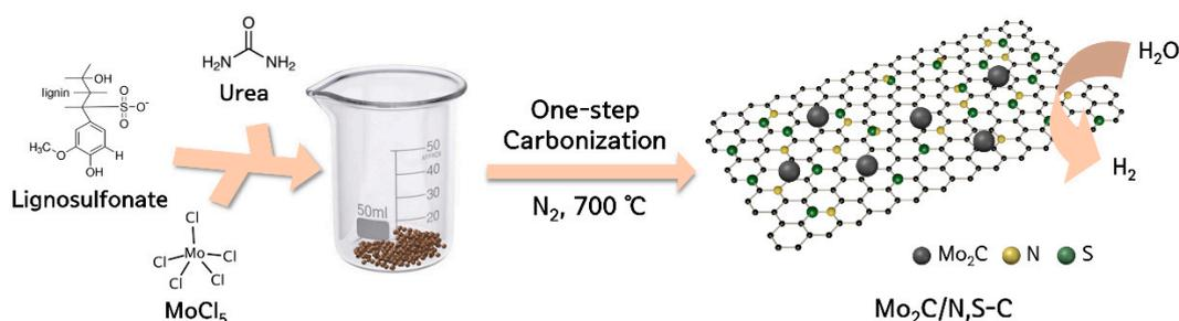
**Scheme 1.** Schematic illustration for the preparation of  $\text{Mo}_2\text{C}/\text{N,S-C}$ .
