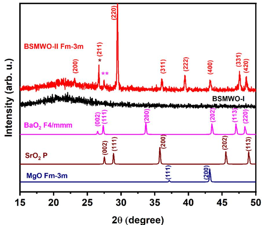
**Figure 1.** XRD patterns of thin films deposited by spin coating and annealed at different temperatures: BSMWO–I—black line, 800 °C, 1 h; BSMWO–I—red line, 800 °C, 1 h and 850 °C, 45 min. XRD patterns are compared with three possible impurity phases that may exist. The XRD peaks noted with \* and \*\* may have contributions from the tetragonal BaO<sub>2</sub> and SrO<sub>2</sub> phases.
