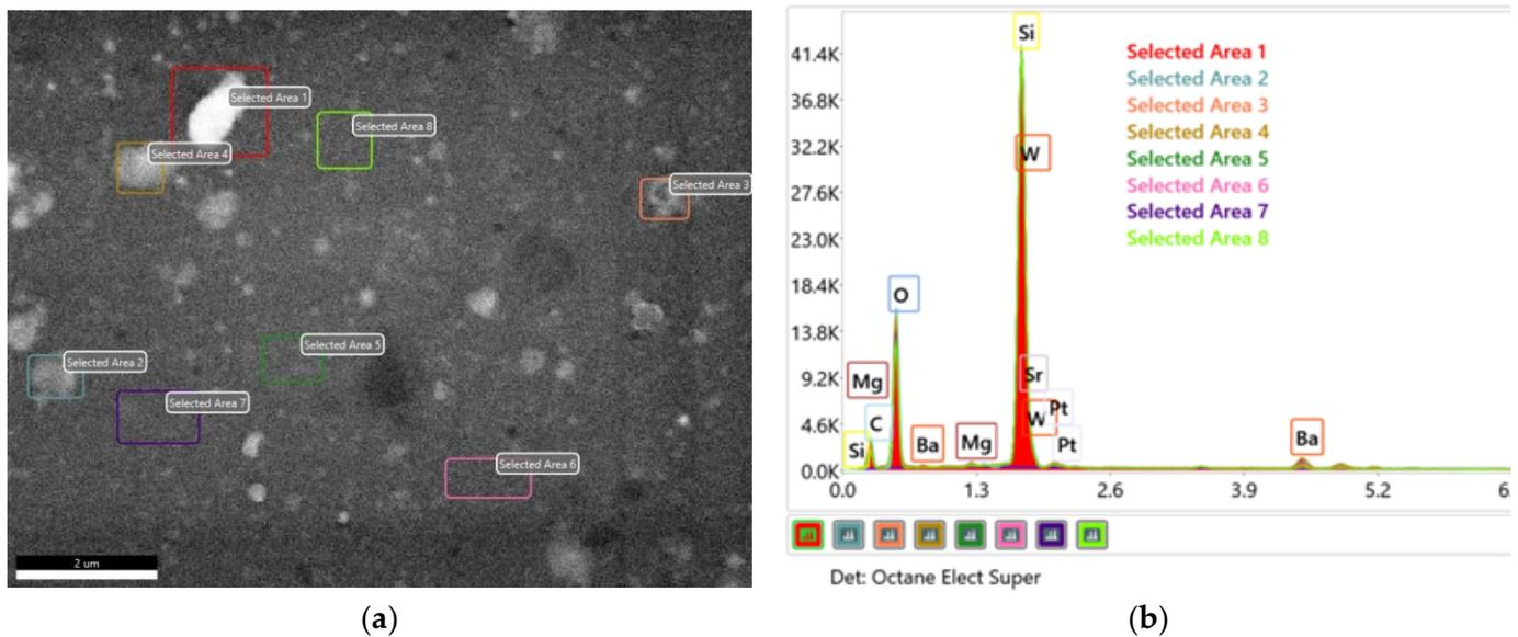
**Figure 3.** EDX spectra belonging to 8 different areas of the BSMWO–II SEM image: (a) SEM image; (b) EDX spectra. The investigated area and the corresponding spectra are marked with the same colors.
