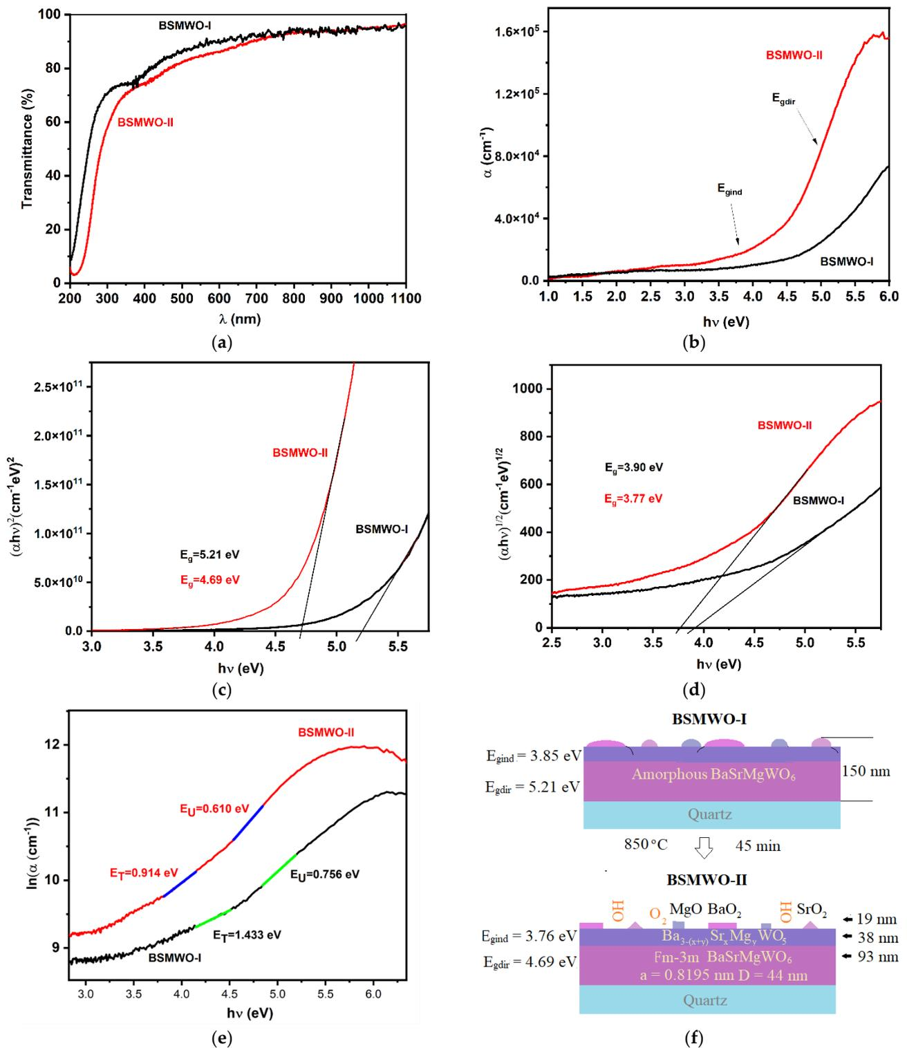
**Figure 5.** Optical properties of BSMWO–I and BSMWO–II thin films: (a) transmittance spectra; (b) absorption coefficient; (c) determination of optical band gap energy for a direct transition; (d) determination of optical band gap energy for an indirect transition; (e) determination of Urbach and UTW energies; (f) thin-film characteristics.
