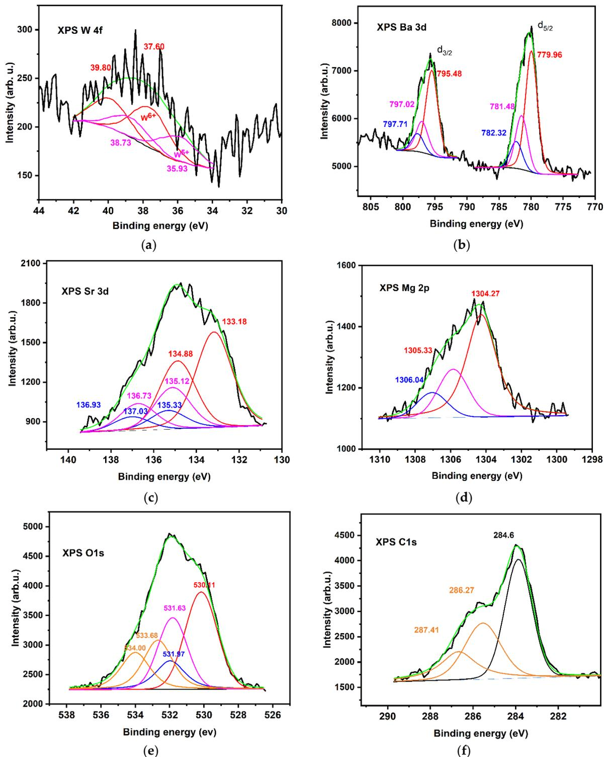
**Figure 4.** High-resolution XPS spectra of BSMWO–II thin film: (a) Ba 3d; (b) Sr 3d; (c) Mg 1s; (d) W 4f; (e) O 1s; (f) C 1s. Red line indicates species in cubic coordination in double perovskite structure, blue line indicates surface species, and orange line indicates adsorbed species.
