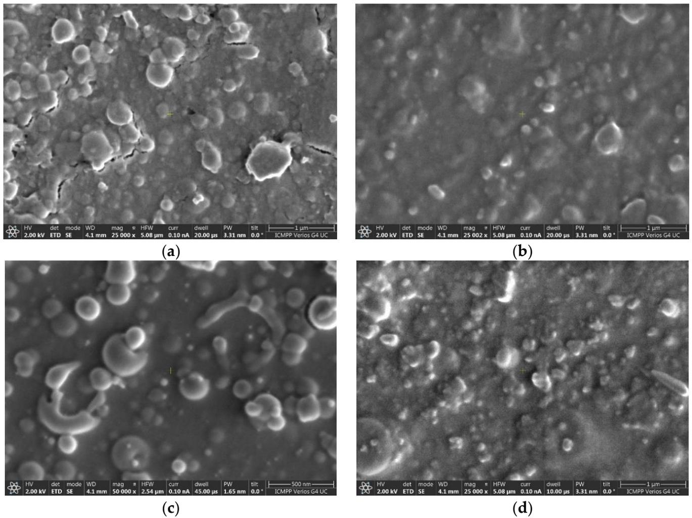
**Figure 2.** SEM images: (a) BSMWO—on quartz substrate; (b) BSMWO—II on quartz substrate; (c) BSMWO—I on (111) Si p substrate; (d) BSMWO—II on (111) Si p substrate.
