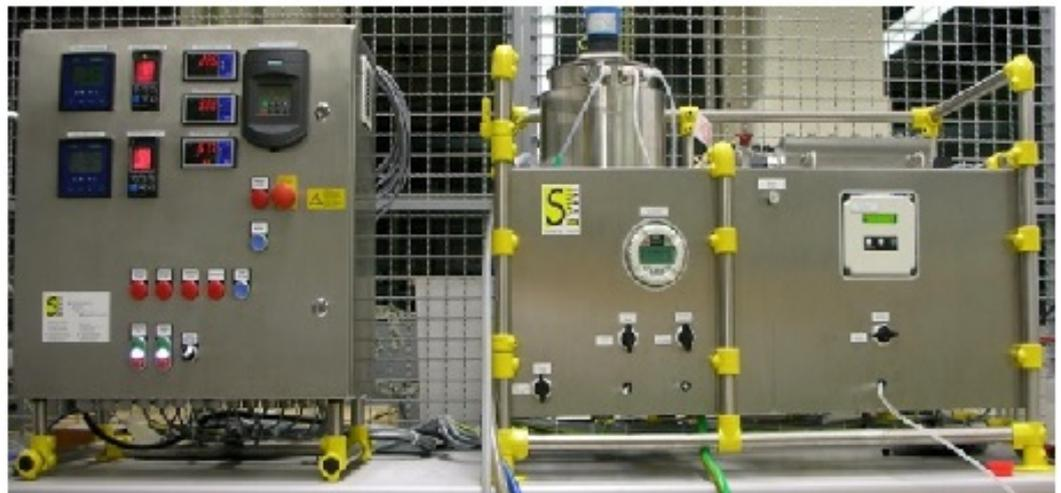
**Figure 2.** Flat sheet membrane test system LSta80.
