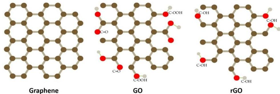
**Figure 3.** The schematic diagram of the structure of graphene, GO, and rGO. Reproduced from ref. [64].
