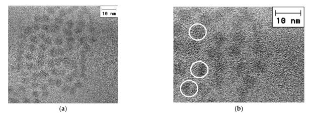
**Figure 5.** (a) HRTEM image of CdSe NCs lying on Si substrate. (b) Zoomed area of HRTEM image (a) with some NCs highlighted by white circles illustrating the crystalline structure of NCs.
