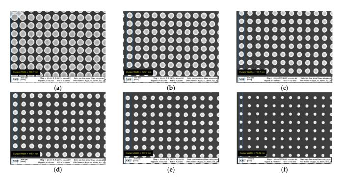
**Figure 1.** Representative high-resolution SEM images of Au nanocluster arrays with a period of 200 nm and various nanocluster diameters: (a) 170 nm, (b) 145 nm, (c) 132 nm, (d) 116 nm, (e) 107 nm, and (f) 74 nm.
