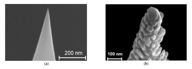
**Figure 4.** (a) SEM image of commercial Si AFM tip (a). (b) SEM image of TERS tip apex covered with Au/Ti.
