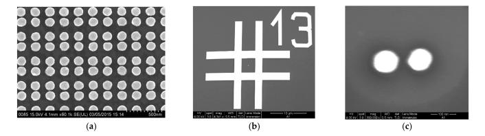
**Figure 2.** (a) Representative high-resolution SEM image of an Au dimer array with a period of 200 nm and a nanodisk diameter of 130 nm. (b) SEM image of a single dimer placed in the center of the cross marked as 13. (c) Zoomed SEM image of single dimer from (b) with nanodisk diameter of 90 nm and a distance (center to center) between nanodisks of 150 nm.
