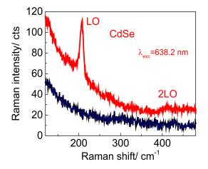
**Figure 7.** SERS spectra of CdSe NC monolayer measured on a Klarite substrate and on the flat gold, red and blue curves, respectively.
