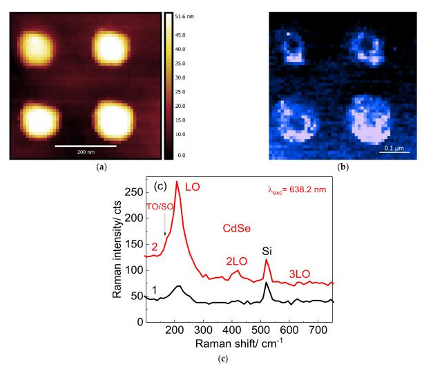
**Figure 12.** (**a**) AFM image of a nanodisk array covered with a monolayer of CdSe NCs, (**b**) TERS map of LO phonon mode from CdSe NCs measured simultaneously with the AFM image shown in (**a**). The most intense TERS signal in the TERS map comes predominantly from edges of Au nanodisks. (**c**) Comparison of the TERS spectra of CdSe NCs measured on the flat Si/SiO<sub>2</sub> substrate (black spectrum 1) and at the corner of a nanodisk (red spectrum 2).
