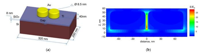
**Figure 10.** Scheme of the model used to calculate the EM enhancement: (**a**) two gold nanodisks formed on a Si surface with an 8 nm thick  $SiO_2$  layer. (**b**) Side-view image of the electric field distribution near the two nanodisks. The electric field near the nanodisks was normalized to the incident electric field. Reprinted with permission from [34]. Copyright 2019, Springer.
