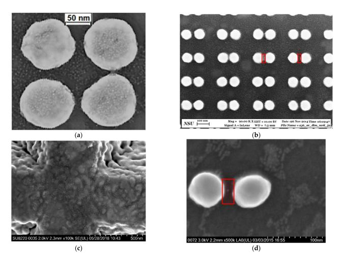
**Figure 6.** SEM images of a fragment of the Au nanodisk array (**a**), dimers (**b**), and Klarite substrate (**c**) covered homogeneously with CdSe NCs (tiny bright spots). (**d**) Typical SEM image of single nanodimer covered by a submonolayer of CdSe NCs. The red semitransparent rectangular areas indicate regions with CdSe NCs contributing to SERS. The images are adapted from [43]. Copyright 2016, Elsevier.
