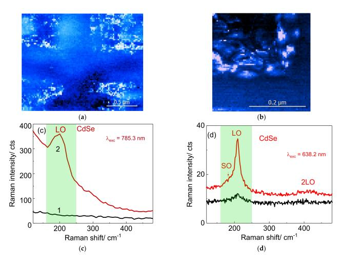
**Figure 8.** TERS mapping of Klarite structure at a wavelength of (**a**) 785.3 nm and (**b**) 638.2 nm. TERS maps indicate the intensity of the LO CdSe mode depending on the position of the tip during the TERS scan. The most intense TERS spectra, red spectra in (**c**,**d**) are taken from the TERS mapping in (**a**,**b**), measured by using 785.3 and 638.2 nm wavelengths, respectively. The black spectra in (**c**,**d**) were taken on a flat part of the gold surface.
