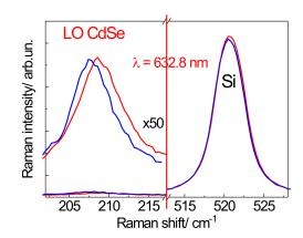
**Figure 11.** SERS spectra measured on two different single dimers reveal the LO phonon feature around 208 cm<sup>-1</sup> and a frequency shift of 1.1 cm<sup>-1</sup>. Si peaks are shown for reference. Adapted with permission from [41]. Copyright 2016, Elsevier.
