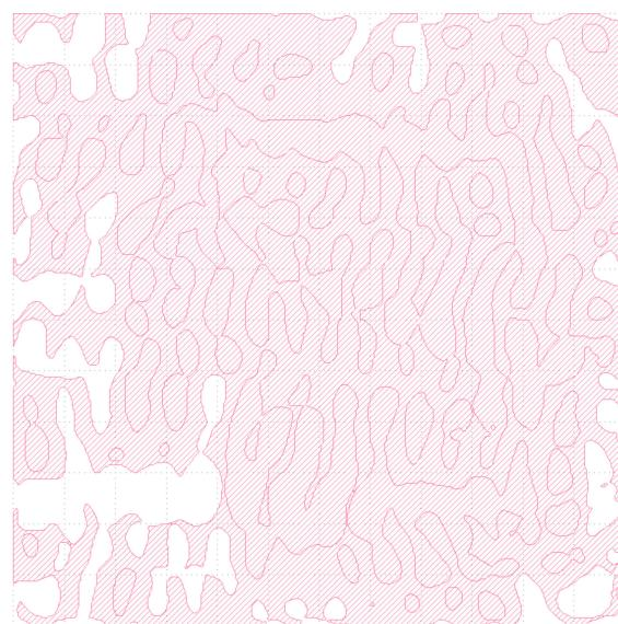
**Figure 12.** GDSII pattern definition for OSU metastructure layout.
