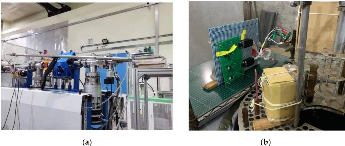
**Figure 1.** The experimental setup of (a) DDD and (b) TID test.
