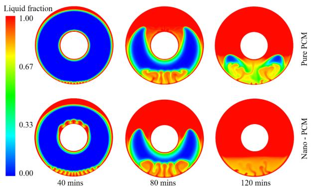
Figure 10. Liquid fraction of PCM during the melting processes with and without nanoparticles.
