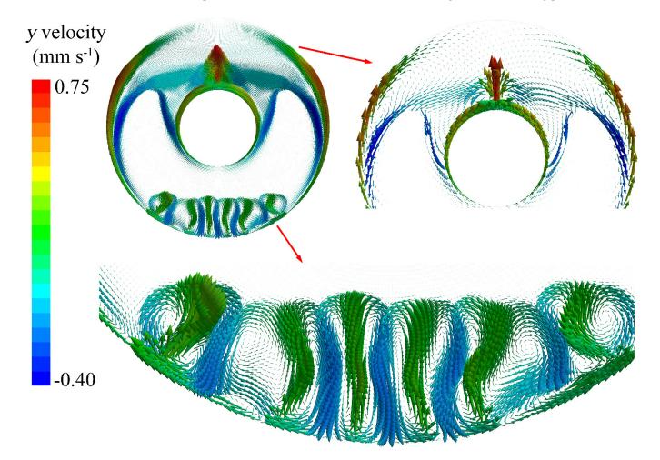
**Figure 8.** *y* velocity vectors during the PCM melting process at t = 85 min.
