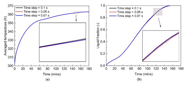
**Figure 4.** Effect of time step on the computational results of the melting process of phase change materials. (a) Average temperature; (b) Liquid fraction.
