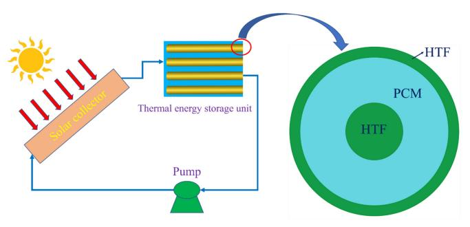
**Figure 1.** Solar energy heating system with a thermal energy storage unit integrated with phase change materials.
