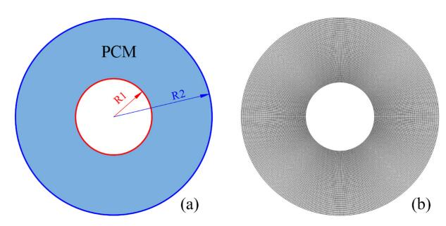
**Figure 2.** Geometry (**a**) and computational mesh (**b**) for the tubular phase change material thermal energy storage unit.
