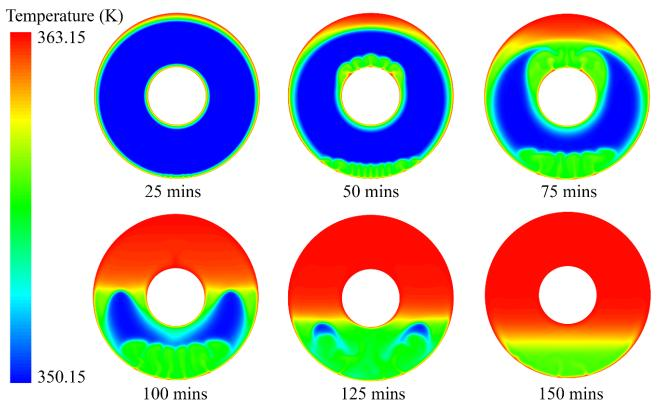
Figure 6. Temperature distribution of PCM during the melting process.
