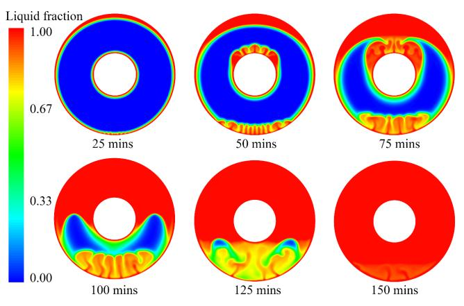
Figure 7. Liquid fraction of PCM during the melting process.
