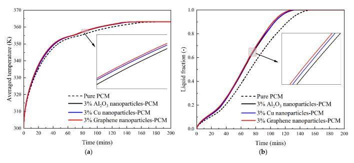
**Figure 12.** Effect of Al<sub>2</sub>O<sub>3</sub>, Cu, Graphene nanoparticles on the melting process of PCM. (**a**) Average temperature; (**b**) Liquid fraction.
