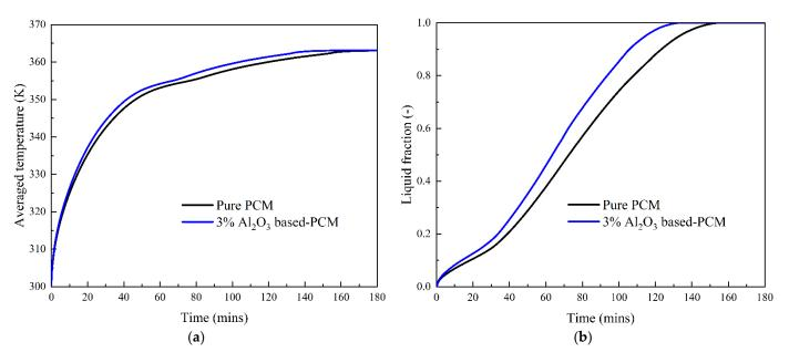
**Figure 11.** Effect of Al<sub>2</sub>O<sub>3</sub> nanoparticles on the PCM melting process. (a) Average temperature; (b) Liquid fraction.
