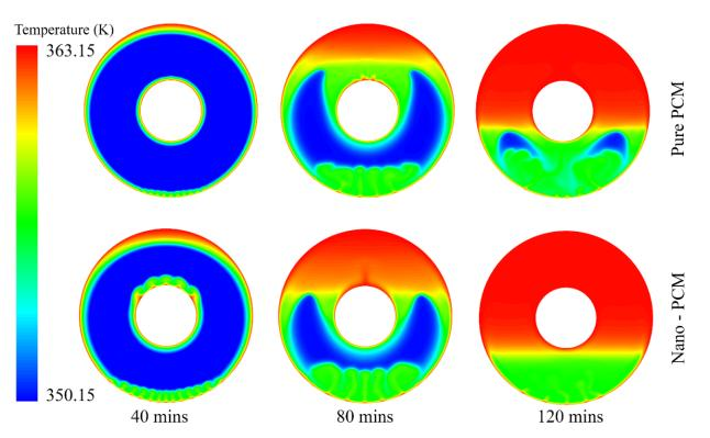
**Figure 9.** Temperature distribution of PCM during the melting processes with and without nanoparticles.
