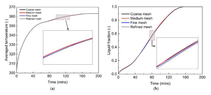
**Figure 3.** Effect of grid density on the computational results of the melting process of phase change materials. (a) Average temperature; (b) Liquid fraction.
