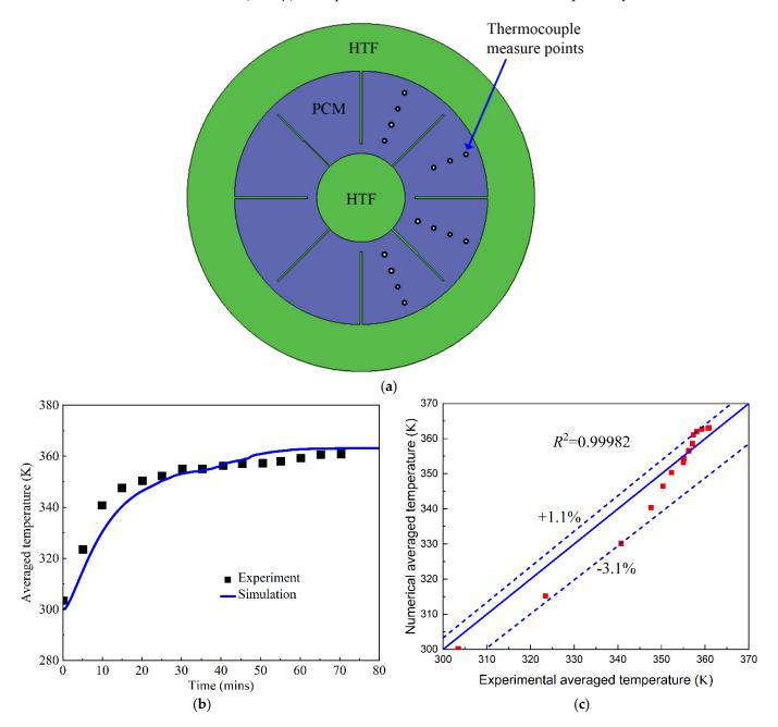
**Figure 5.** Model validation of the melting process of phase change materials. (**a**) Thermocouple measure points in the experiments [32]; (**b**) Average temperature; (**c**) Error analysis.
