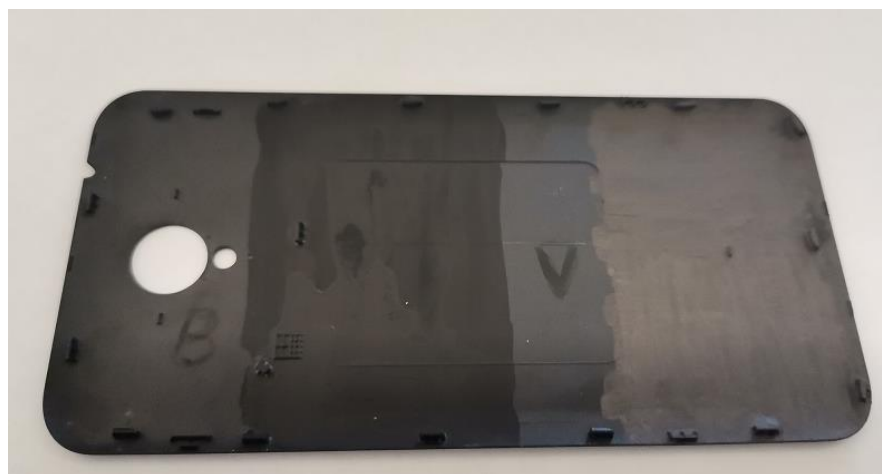
Figure 12. Cellular phone back side chassis coated with 2 paints samples.
