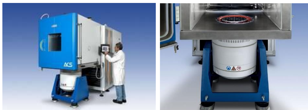
Figure 2. Angelantoni CH250 climatic chamber + TIRA S55240/LS—Vibration system.
