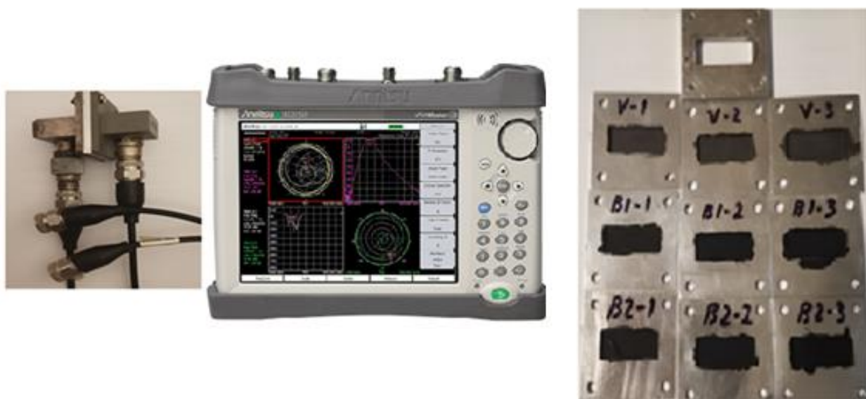
Figure 1. The measuring setup for EMI-shielding efficiency based on the ANRITSU Vector Network Analyzer.
