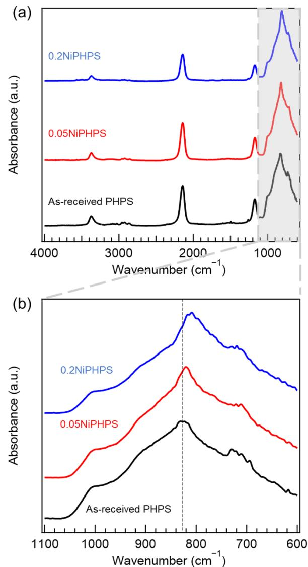
**Figure 1.** ATR-FTIR spectra of as-received PHPS (black line) and Ni-modified PHPS samples (red and blue lines represent the Ni/Si atomic ratios of 0.05 and 0.2, respectively): (a) 600–4000 cm<sup>-1</sup> and (b) 600–1100 cm<sup>-1</sup>.
