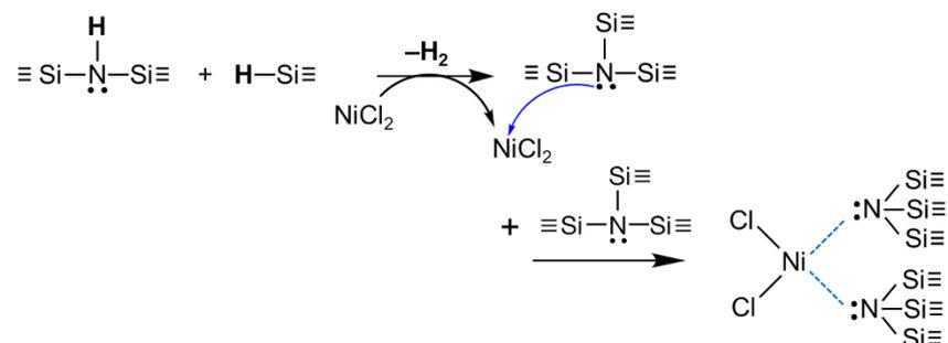
**Scheme 1.** Dehydrogenation reaction of Si-H/N-H in PHPS catalyzed by NiCl<sub>2</sub> and possible Ni(II) coordination structures, such as 4-coordinate Ni(II) complex.
