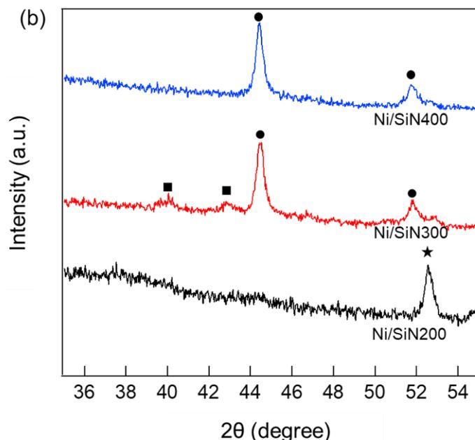
**Figure 3.** Powder X-ray diffraction patterns of Ni/SiN<sub>x</sub> samples pyrolyzed at 200, 300, 400 °C: 2θ = (a) 10–90° and (b) 35–55°.
