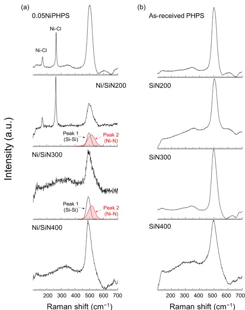
**Figure 4.** Raman spectra of (a) 0.05NiPHPS and Ni/SiNX and (b) as-received PHPS and SiNX samples. Deconvolution by the Gaussian curve fitting performed on the broad peak around  $500\text{ cm}^{-1}$  detected for the Ni/SiN200 and Ni/SiN300 samples yielded two peaks centered at  $495$  and  $515\text{ cm}^{-1}$  labeled as **Peak 1** and **Peak 2**, respectively.
