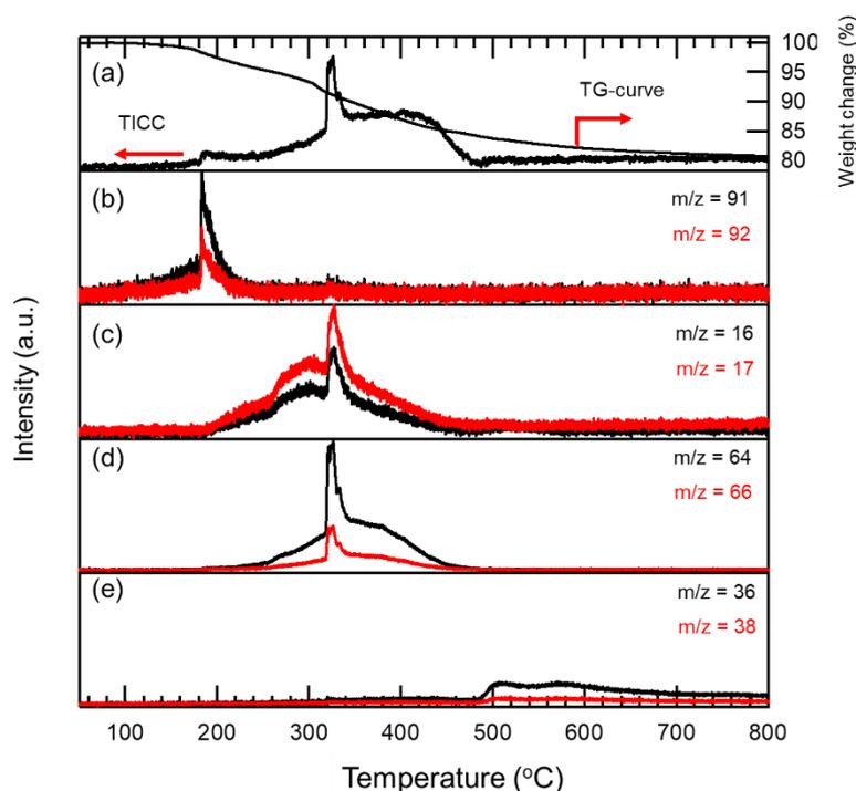
**Figure 2.** TG-MS analysis under flowing He of the 0.05NiPHPS sample: (a) TG-curve coupled with the total ion current chromatogram (TICC), (b–e) the simultaneous monitoring of gaseous products formed in situ.
