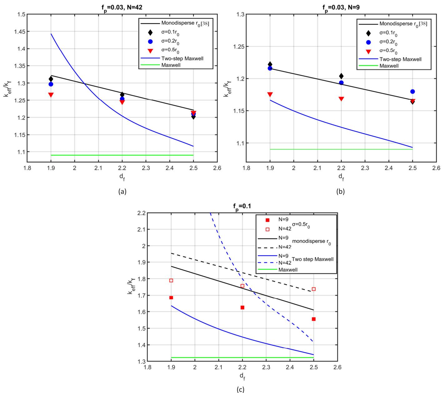
**Figure 4.** Effective thermal conductivity as a function of fractal dimension for: (a) volume fraction  $f_p = 0.03$  and number of particles per aggregate  $N = 42$ ; (b)  $f_p = 0.03$ ,  $N = 9$ ; (c)  $f_p = 0.1$ ,
