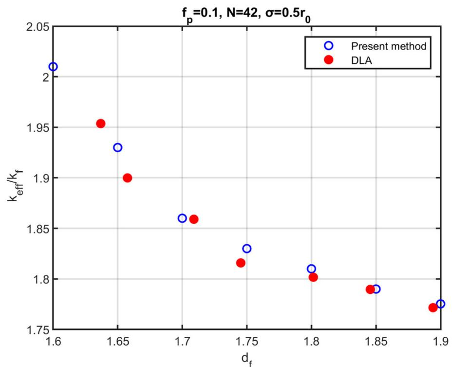
**Figure 3.** Effective thermal conductivity as a function of the fractal dimension of aggregates consisting of polydispersed particles by the present method (open, blue symbols) and by simulations from the DLA method (filled, red symbols).
