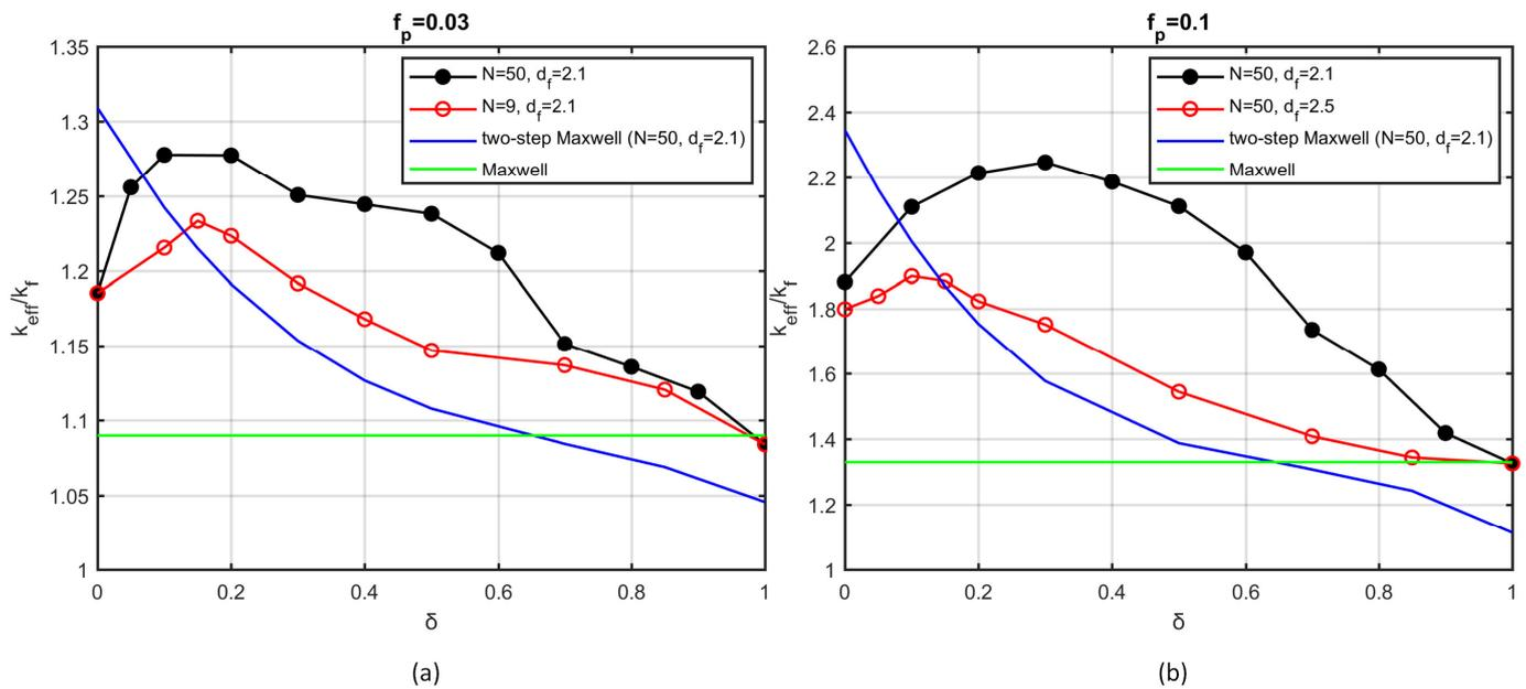
**Figure 5.** Effective thermal conductivity as a function of overlapping coefficient: (a) volume fraction  $f_p = 0.03$ ; (b) volume fraction  $f_p = 0.1$ . Solid, black circles:  $N = 50, d_f = 2.1$ . Open, red circles: (a)  $N = 9, d_f = 2.1$ ; (b)  $N = 50, d_f = 2.5$ . Blue lines: two-step Maxwell model. Green lines: Maxwell model.
