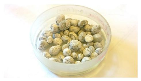
Figure 2. Granules of unsintered sorbent.
