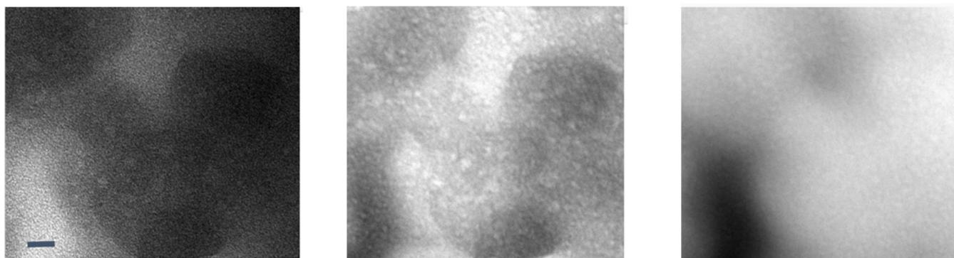
**Figure 6.** Low-loss EFTEM image series of a soluble fullerene/polyethylene oxide-based lithium-conducting solid electrolyte. From left to right: 0 eV, 30 eV, and 62 eV. The images show fullerene aggregates (white dots) with the highest contrast at an energy loss of 30 eV. These are unpublished images related to the work published in [79]. The scale bar is 10 nm.
