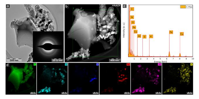
**Figure 2.** (a) HRTEM image of a C-Flax sample. (b) Darkfield HRTEM image used for EDS chemical mapping. (c) EDAX spectrum of C-Flax sample. (d) EDS elemental mapping of C-Flax sample, including carbon, nitrogen, oxygen, iron, aluminum, and potassium atoms. Scale bars were unified from the graphical point-of-view to provide better visibility.
