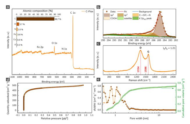
**Figure 1.** (a) XPS survey spectrum of C 1s, N 1s, O 1s, and Fe 2p with related atomic % weight contributions (inset). (b) Deconvoluted C 1s peak. (c) Raman spectrum of C-Flax sample. (d) Adsorption/desorption isotherm of C-Flax sample and its (e) related pore size distribution and cumulative pore volume.
