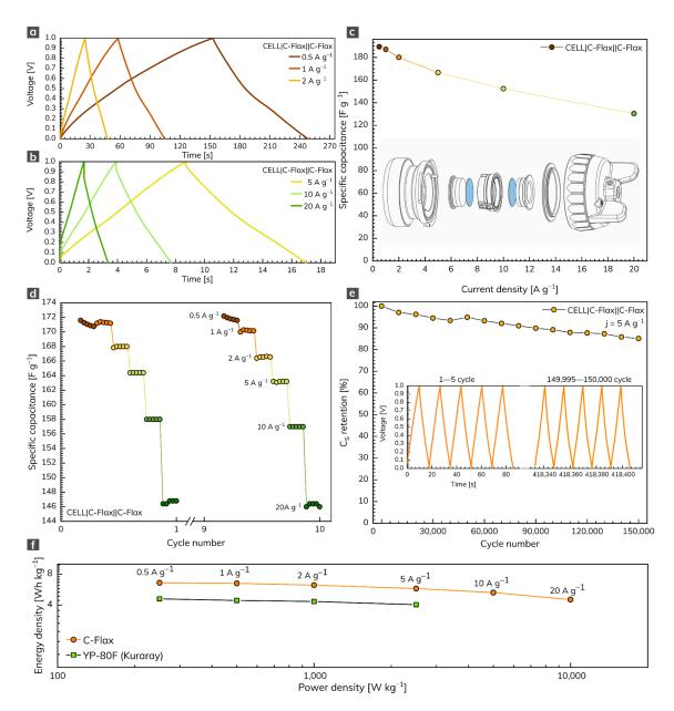
**Figure 4.** (**a**,**b**) GCD profiles of C-Flax material recorded at different current densities and (**c**) corresponding specific capacitance vs. current density profile. (**d**) Rate-test of C-Flax sample recorded at current densities ranging from 0.5 to 20 A  $g^{-1}$ . (**e**) Specific capacitance retention of C-Flax sample after 150,000 GCD cycles. (**f**) Ragone plot of C-Flax and YP-80F (Kuraray) sample. All experiments were performed in 1 mol L<sup>-1</sup> sulfuric acid.
