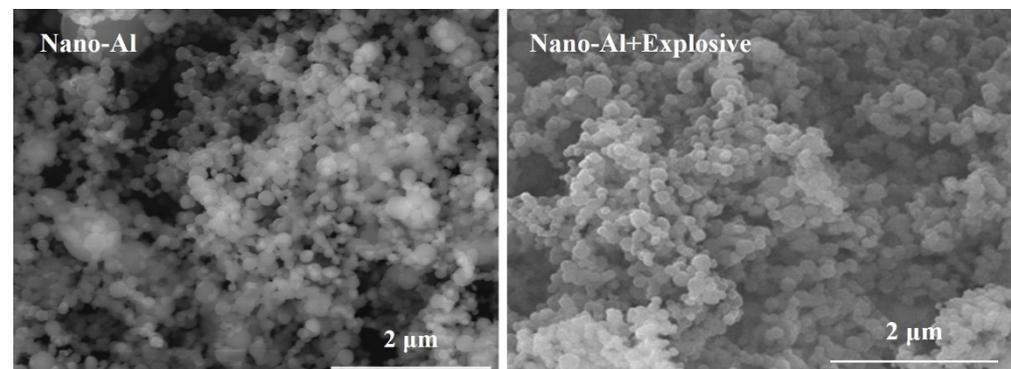
**Figure 6.** SEM images of nano-Al and explosive containing nano-Al.
