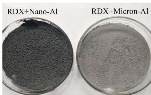
**Figure 2.** Photography of RDX with Nano-Al and Micron-Al.
