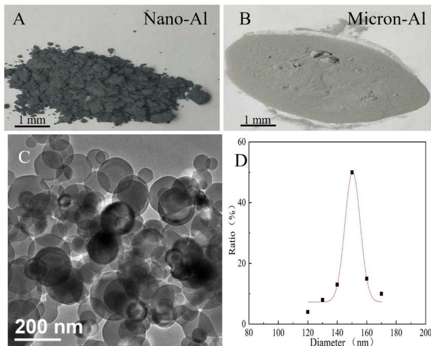
**Figure 1.** Photography of nano-Al (A) and micron-Al (B) powders. (C) TEM tests of nano-Al and (D) the distribution of the diameter of nano-Al powder.
