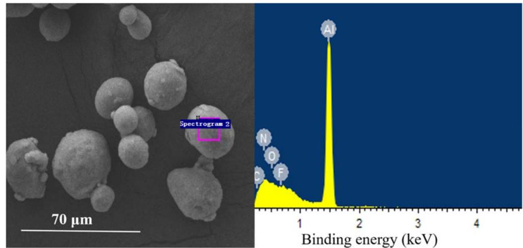
**Figure 5.** SEM image and EDS spectra of explosive 2.
