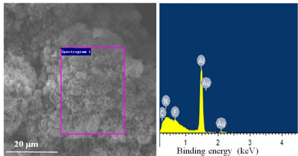
Figure 4. SEM image and EDS spectra of explosive 1.
