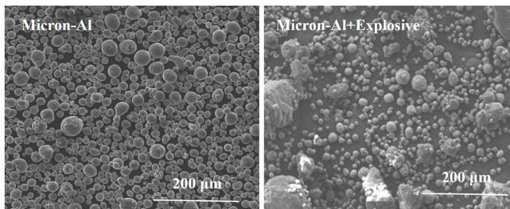
**Figure 7.** SEM images of micron-Al and explosive containing micron-Al.
