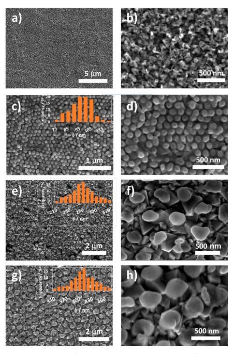
**Figure 3.** SEM top images of an iron oxide compact layer (**a**,**b**) synthesized by e-beam evaporation directly on a FTO substrate, and iron oxide nanopillars synthesized by e-beam evaporation using AAO templates with different diameters:  $\varphi$ 90 nm (**c**,**d**),  $\varphi$ 260 nm (**e**,**f**) and  $\varphi$ 400 nm (**g**), (**h**) on FTO substrates.
