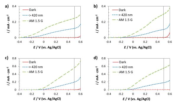
Figure 5. Current/photocurrent density versus applied potential curves of the photoanodes fabricated on FTO substrates: compact layer (a) and using different AAO templates:  $\varphi$ 90 nm (b),  $\varphi$ 260 nm (c) and  $\varphi$ 400 nm (d). Dark, visible light ( $\lambda$  > 420 nm) and solar AM 1.5 G (55 mW·cm<sup>-2</sup>) illumination conditions were applied.
