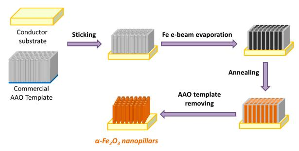
**Figure 2.** Schematic representation of the experimental procedure to fabricate self-standing  $\alpha$ -Fe<sub>2</sub>O<sub>3</sub> nanopillars with controllable diameters, by using e-beam evaporation technique with AAO templates.
