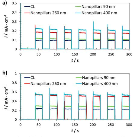
Figure 7. Chopped-light chronoamperometry measurements at 0.5 V (vs. Ag/AgCl) of the photoanodes fabricated on FTO substrates, under visible light ( $\lambda > 420$  nm) (a) and under solar AM 1.5 G ( $55 \text{ mW} \cdot \text{cm}^{-2}$ ) illumination (b).
