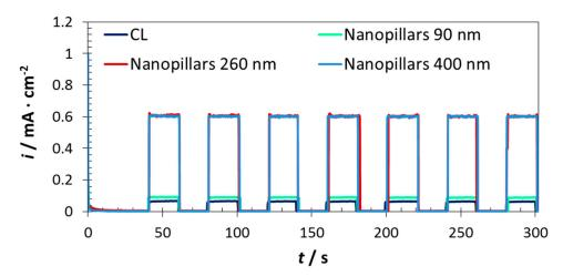
**Figure 8.** Chopped-light chronoamperometry measurements at 0.5 V (vs. Ag/AgCl) of the photoanodes fabricated on Ti substrates, under visible light ( $\lambda > 420$  nm).
