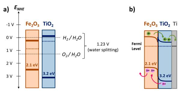
Scheme 1. Energy bands positions of Fe<sub>2</sub>O<sub>3</sub> and TiO<sub>2</sub> semiconductors when isolated (a) and when they are connected (b).
