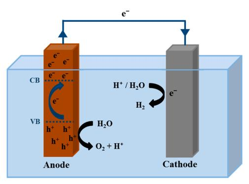
Figure 1. Schematic representation of a PEC cell.
