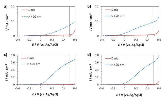
**Figure 6.** Current/photocurrent density versus applied potential curves of the photoanodes fabricated on Ti substrates: compact layer (a) and using different AAO templates:  $\varphi$ 90 nm (b),  $\varphi$ 260 nm (c) and  $\varphi$ 400 nm (d). Dark and visible light ( $\lambda$  > 420 nm).
