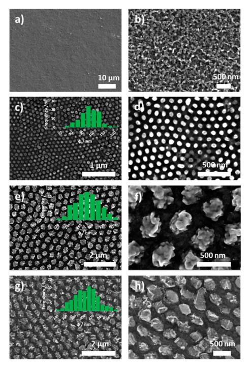
**Figure 4.** SEM top images of an iron oxide compact layer (**a**,**b**) synthesized by e-beam evaporation directly on a Ti foil, and iron oxide nanopillars synthesized by e-beam evaporation using AAO templates with different diameters:  $\varphi$ 90 nm (**c**,**d**),  $\varphi$ 260 nm (**e**,**f**) and  $\varphi$ 400 nm (**g**,**h**) on Ti foils.
