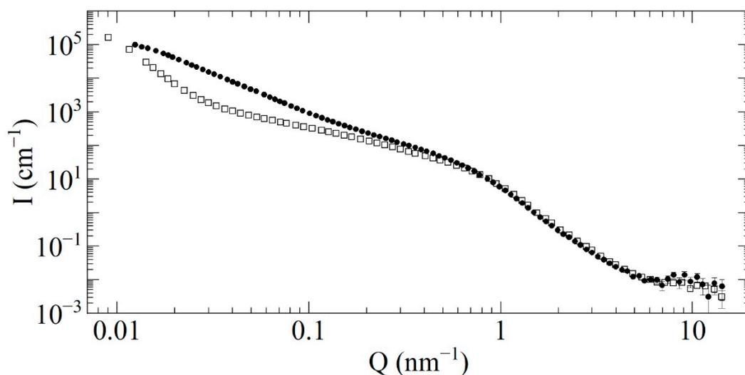
**Figure 6.** The intensity  $I \text{ (cm}^{-1}\text{)}$  of scattering versus the neutron-transferred momentum  $Q \text{ (nm}^{-1}\text{)}$  for the F-DNDs (solid circles) and DF-DNDs (open squares). Both curves are normalized to the equal sample density of  $0.19 \text{ g/cm}^3$ .
