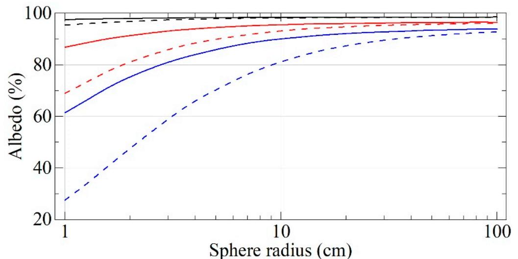
**Figure 12.** Neutron albedo for the velocities of 50 m/s (black lines), 100 m/s (red lines), and 150 m/s (blue lines) for F-DNDs (dashed lines) and DF-DNDs (solid lines) versus the cavity radius. The incident neutrons are isotropic, the powder thickness is infinite, and densities of F-DNDs and DF-DNDs are equal to 0.19 and 0.56 g/cm<sup>3</sup>, respectively.
