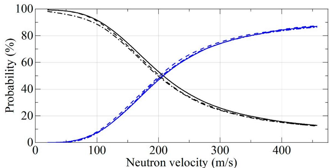
**Figure 11.** The probability of neutron reflection (black lines) and transmission (blue lines) for F-DNDs (dashed lines) and DF-DNDs (solid lines) and DNDs (dash-dotted lines) versus neutron velocity. The probability of neutron absorption is below 1% for F-DNDs and DF-DNDs at any velocity and 1–5% for DNDs. The incident neutrons are isotropic, the powder density is  $0.19 \text{ g/cm}^3$ , and the powder layer thickness is 3 cm.
