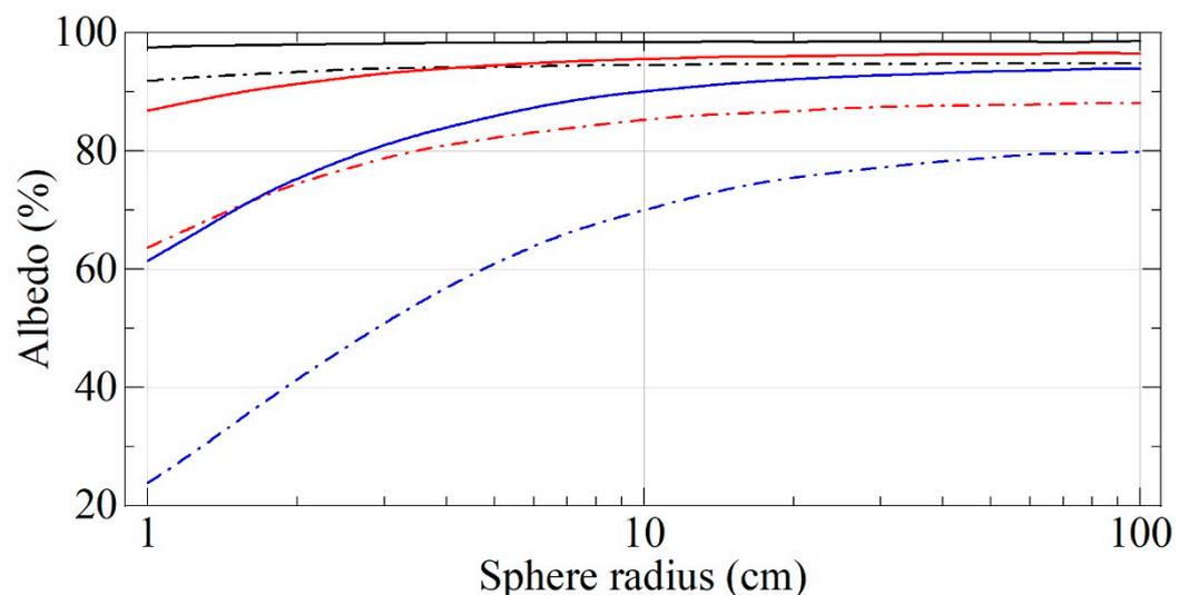
**Figure 13.** Neutron albedo for the velocities of 50 m/s (black lines), 100 m/s (red lines), and 150 m/s (blue lines) for DF-DNDs (solid lines) and DNDs (dash-dotted lines) versus the cavity radius. The incident neutrons are isotropic; the powder thickness is infinite. DF-DNDs density is equal to 0.56 g/cm<sup>3</sup>. The DNDs density is the same as it is in Figure 12 and equal to 0.19 g/cm<sup>3</sup>.
