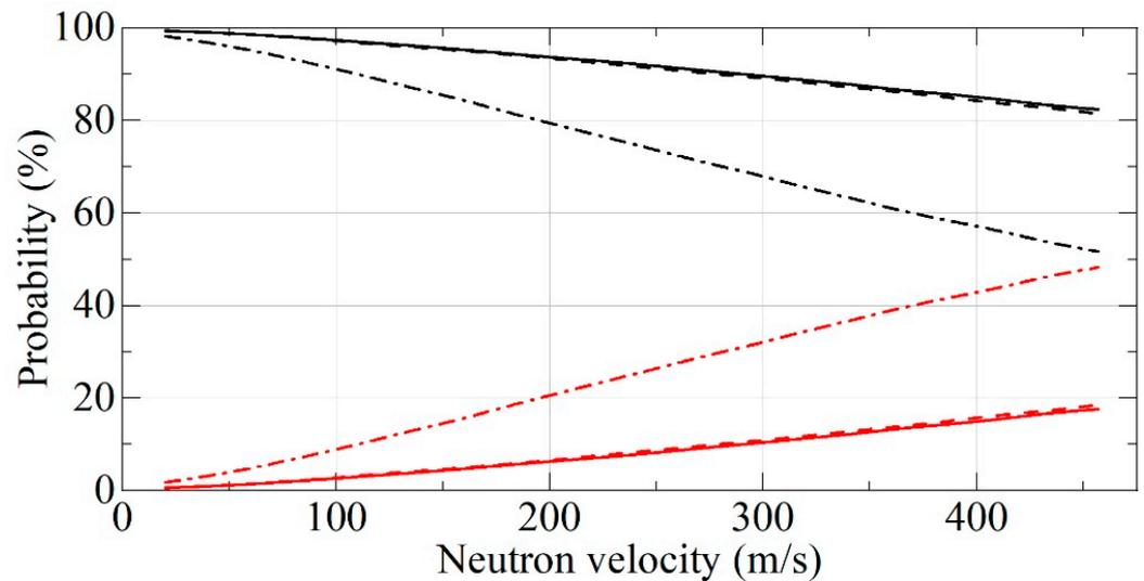
**Figure 10.** The probability of neutron reflection (black lines) and absorption (red lines) for F-DNDs (dashed lines) and DF-DNDs (solid lines) and DNDs (dash-dotted lines) versus neutron velocity. The incident neutrons are isotropic, the powder density is  $0.19 \text{ g/cm}^3$ , and the powder thickness is infinite.
