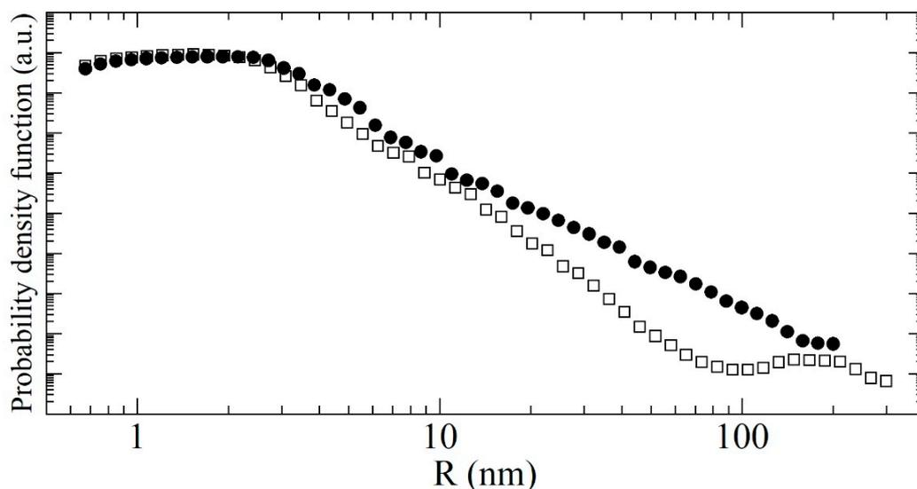
**Figure 8.** The probability density versus radius (in nm) calculated with the discrete-sized diamond nanospheres model for the F-DNDs (solid circles) and DF-DNDs (open squares). Points correspond to the results of calculation.
