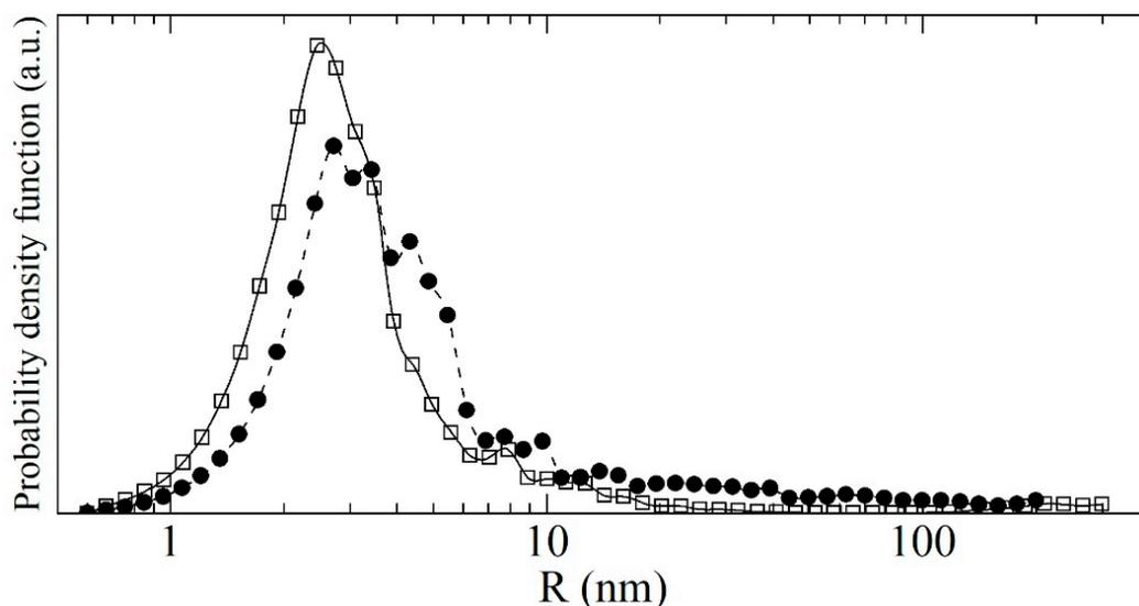
**Figure 9.** The log-linear volume distribution of scatterers evaluated using the discrete-sized diamond nanospheres model for the F-DNDs (solid circles) and DF-DNDs (open squares). Solid (DF-DNDs) and dashed (F-DNDs) lines interpolate the calculated results.
