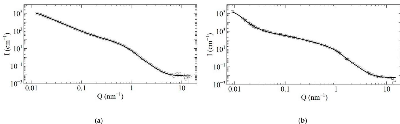
**Figure 7.** Comparison of measured (open circles and squares) and simulated (solid lines) scattering intensity  $I$  ( $\text{cm}^{-1}$ ) versus the neutron-transferred momentum  $Q$  ( $\text{nm}^{-1}$ ): (a) F-DND; (b) DF-DND samples.
