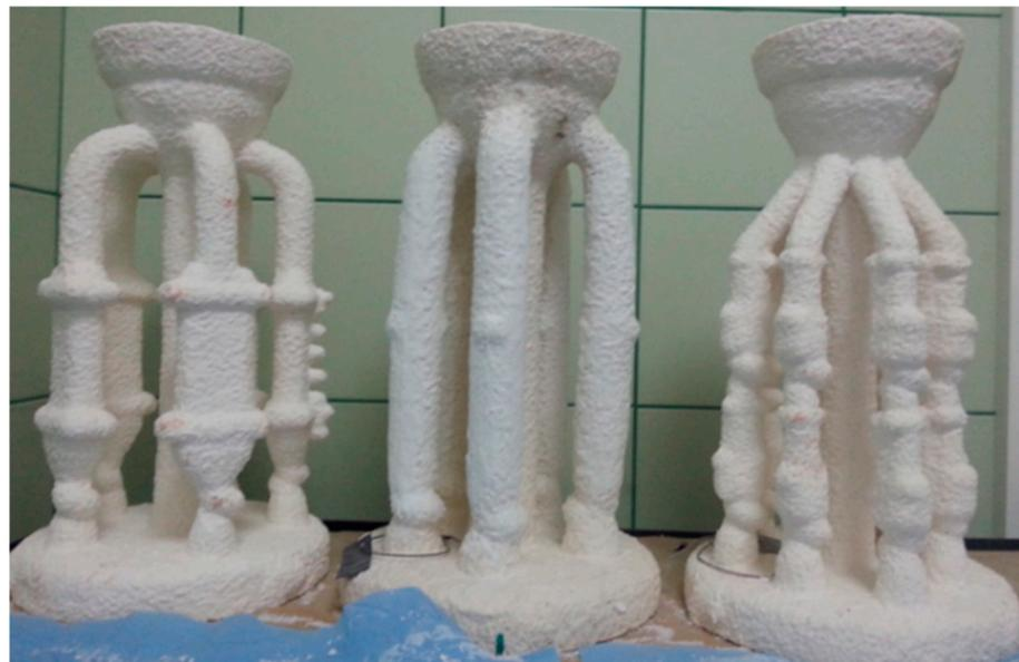
Figure 19. Examples of corundum ceramic moulds obtained with Ludox AM and Remasol binders.
