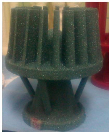
**Figure 3.** Example SiC mould (raw state) obtained using Imerys W440 binder.
