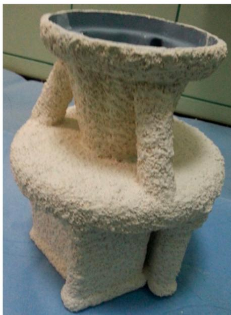
**Figure 20.** Example of a  $ZrO_2$  ceramic mould obtained with Ludox SK and EHT binders.
