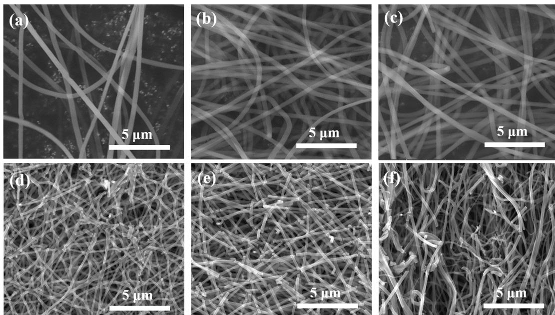
Figure 10. FE-SEM images of PVP/TiO<sub>2</sub> nanofibers with different fluid velocities before (a) 0.1 mL/h, (b) 0.5 mL/h, (c) 1.0 mL/h and after heat treatment (d) 0.1 mL/h, (e) 0.5 mL/h, (f) 1.0 mL/h.
