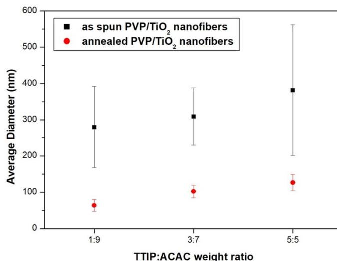
**Figure 13.** Average diameter of PVP/TiO<sub>2</sub> nanofibers with different weight ratios of TTIP and ACAC before and after heat treatment.
