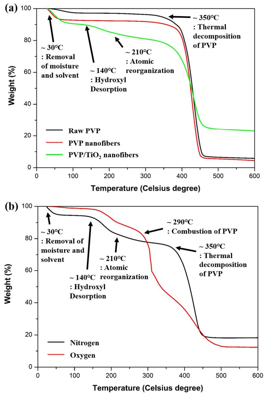
**Figure 8.** TGA curves of (a) raw PVP, PVP nanofibers, PVP/TiO<sub>2</sub> nanofibers in a nitrogen atmosphere, and (b) PVP/TiO<sub>2</sub> nanofibers in a nitrogen and oxygen atmosphere.
