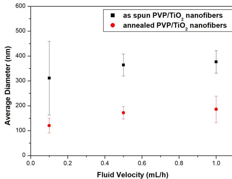
**Figure 11.** Average diameter of PVP/TiO<sub>2</sub> nanofibers with different fluid velocities before and after heat treatment.
