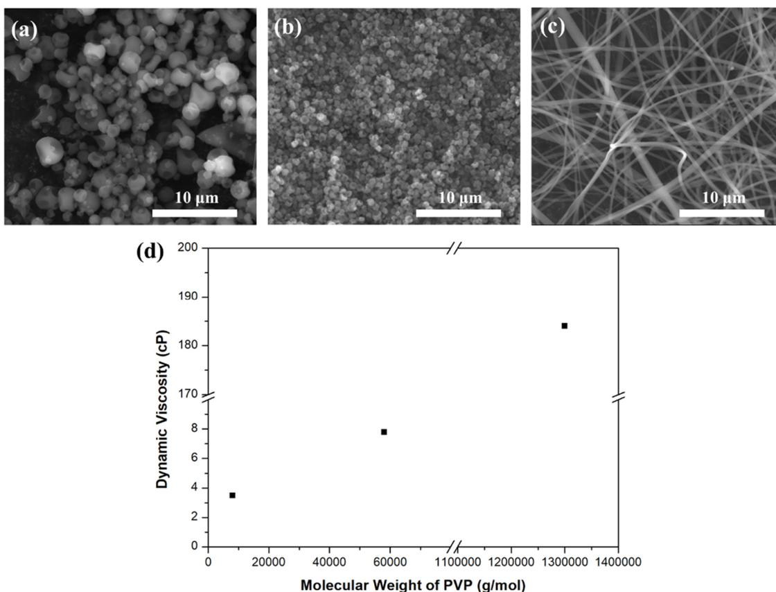
**Figure 1.** FE-SEM images of nanoparticles and nanofibers with different PVP molecular weights: (a) 8000 g/mol, (b) 58,000 g/mol, (c) 1,300,000 g/mol, and (d) dynamic viscosity.
