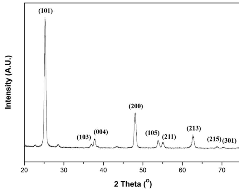
Figure 9. XRD spectrum of heat-treated PVP/TiO<sub>2</sub> nanofibers.
