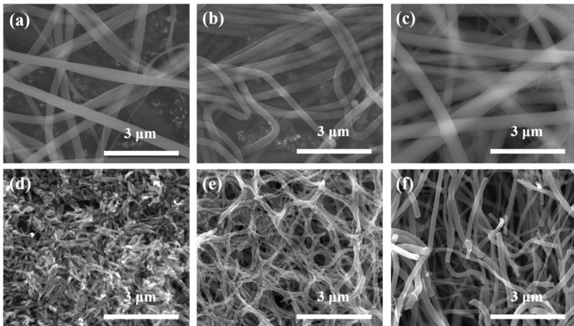
**Figure 12.** FE-SEM images of PVP/TiO<sub>2</sub> nanofibers with different weight ratios of TTIP and ACAC before (a) 1:9, (b) 3:7, (c) 5:5 and after annealing (d) 1:9, (e) 3:7, (f) 5:5.
