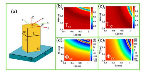
**Figure 1.** (a) Schematic of the Si nanobrick with the rotation angle  $\theta$ . The transmittances (**b**,**c**) and the propagation phases (**d**,**e**) under XLP (**b**,**d**) and YLP (**c**,**e**) incidences of the irrotational Si nanobricks as a function of L and W.
