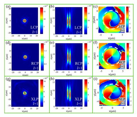
**Figure 5.** The intensity distributions of the vortex beam at the focusing plane under the LCP (**a**), RCP (**d**) and XLP (**g**) light illuminations. The intensity distributions of the converged vortex beam at the x-z plane under the LCP (**b**), RCP (**e**) and XLP (**h**) light illuminations. The phase distributions of the vortex beam at the focusing plane under the LCP (**c**), RCP (**f**) and XLP (**i**) light illuminations.
