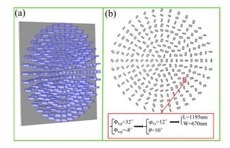
**Figure 2.** (a) Schematic of the spin-selected vortex metalens. (b) Top view of spin-selected vortex metalens, and the designing concept and specific parameters' selection of a unit cell.
