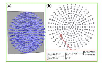
**Figure 4.** (a) Schematic of the spin-independent vortex metalens. (b) Top view of spin-independent vortex metalens, and the designing concept and specific parameters' selection of a unit cell.
