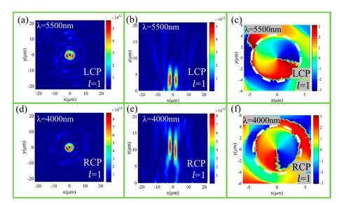
**Figure 6.** The intensity distributions of the vortex beam at the focusing plane under the LCP (5500 nm) (**a**) and RCP (4000 nm) (**d**) light illuminations. The intensity distributions of the converged vortex beam at the x-z plane under the LCP (5500 nm) (**b**) and RCP (4000 nm) (**e**) light illuminations. The phase distributions of the vortex beam at the focusing plane under the LCP (5500 nm) (**c**) and RCP (4000 nm) (**f**) light illuminations.
