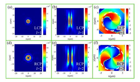
**Figure 3.** The intensity distributions of the vortex beam at the focusing plane under the LCP (**a**) and RCP (**d**) light illuminations. The intensity distributions of the converged vortex beam at the x-z plane under the LCP (**b**) and RCP (**e**) light illuminations. The phase distributions of the vortex beam at the focusing plane under the LCP (**c**) and RCP (**f**) light illuminations.
