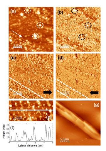
**Figure 5.** DMA-loaded u-PPO400. (a) Contact-mode AFM topography; color-scale range: 64 nm. (b) Ultrasonic force microscopy (UFM) image, recorded simultaneously with (a). (c,d) Lateral Force Microscopy (LFM) images recorded scanning (c) from left to right, and (d) from right to left. (e) Contact-mode AFM topography; color-scale range: 55 nm. (f) Height-contour profile along the continuous white line in (e). (g) Contact-mode AFM topography; color-scale range: 2 µm.
