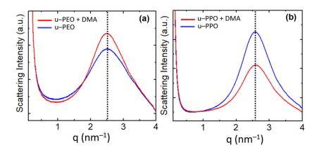
**Figure 7.** Experimental SAXS intensity *I*(*q*) of (**a**) unloaded u-PEO 500 (blue curve) and DMA-loaded u-PEO500 (red curve) and (**b**) unloaded u-PPO (blue curve) and DMA-loaded u-PPO400 (red curve).
