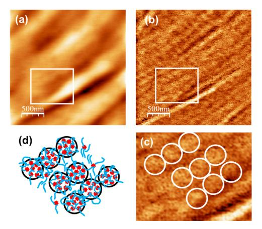
**Figure 8.** Unloaded u-PPO400. (a) Contact-mode AFM topography; color-scale range: 64 nm (b) Ultrasonic force microscopy (UFM) image, recorded simultaneously with (a); (c) Cropping of the part of (b) indicated by the white rectangle (d) Schematic drawing to illustrate the nanostructural arrangement within the polymer matrix.
