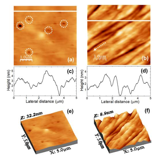
**Figure 3.** (**a**,**b**) Contact mode AFM topographic images of (**a**) unloaded u-PEO500 and (**b**) unloaded u-PPO400 films. (**c**,**d**) Height-contours profiles along the white lines in (**a**,**b**), respectively. (**e**,**f**) 3D representations of (**a**,**b**), respectively.
