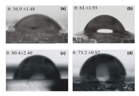
**Figure 10.** Contact-angle measurements on (**a**) unloaded u-PEO500; (**b**) DMA-loaded u-PEO500; (**c**) unloaded u-PPO400; (**d**) DMA-loaded u-PPO400. The results are expressed as the mean  $\pm$  S.D. for n = 3 (replicates).
