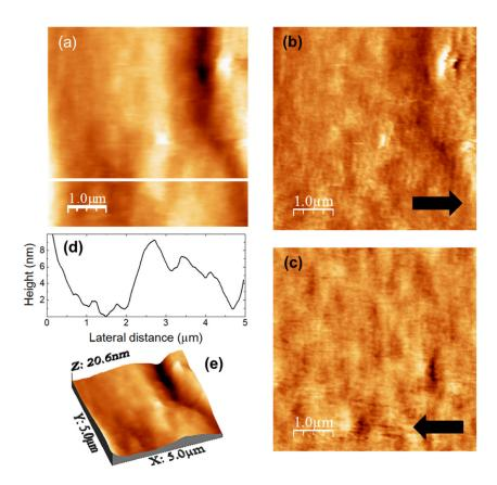
**Figure 4.** DMA-loaded u-PEO500. (**a**) Contact-mode AFM topography. (**b**,**c**) Lateral force microscopy (LFM) images recorded scanning (**b**) scanning from left to right (simultaneously with (**a**)) and (**c**) from right to left. (**d**) Height-contour profile along the continuous white line in (**a**). (**e**) 3D representation of (**a**).
