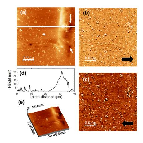
**Figure 11.** u-PPO500 film after DMA release in medium. (a) Contact-mode AFM topography; colorscale range: 35 nm. (b,c) Lateral force microscopy (LFM) images recorded (b) Scanning from left to right (simultaneously with (a)) and (c) from right to left. (d) Height-contours profile along the continuous white line in (a). (e) 3D representation of (a).
