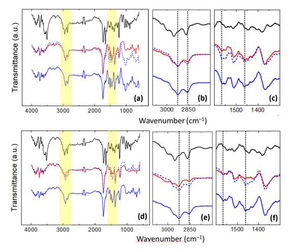
**Figure 9.** FT-IR spectra of (**a**–**c**) pure u-PEO 500 films (blue curves), DMA loaded u-PEO films (red curves) and DMA powder (black curves); and (**d**–**f**) pure u-PPO400 films (blue curves), DMA loaded u-PPO films (red curves) and DMA powder (black curves). In each plot, the dashed blue curve is identical to the continuous blue line and has been shifted vertically to facilitate the comparison of the unloaded and DMA-loaded films' spectra.
