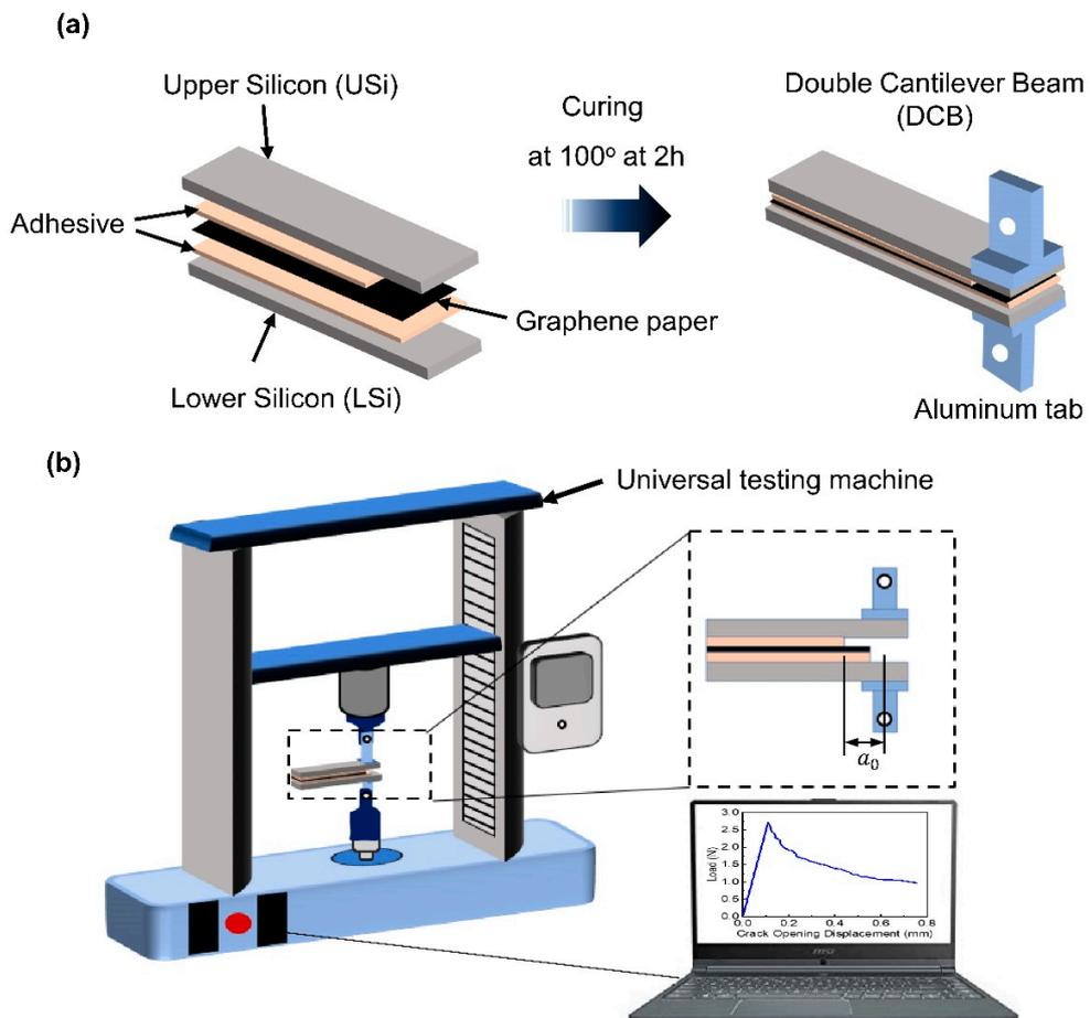
**Figure S3.** Schematic illustration of the mode I fracture tests of the EEG paper: (a) Preparation of the DCB specimen using the EEG paper. (b) Mechanical separation of the EEG paper using a universal testing machine.
