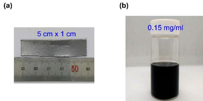
**Figure S2.** Photograph of (a) graphite foils and (b) dispersed EEG flakes in DMF.
