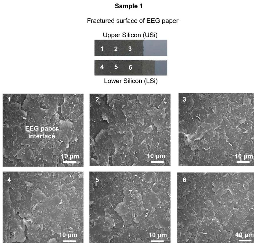
**Figure S5.** SEM images of the fracture surfaces of the upper and lower Si strips after the fracture tests.
