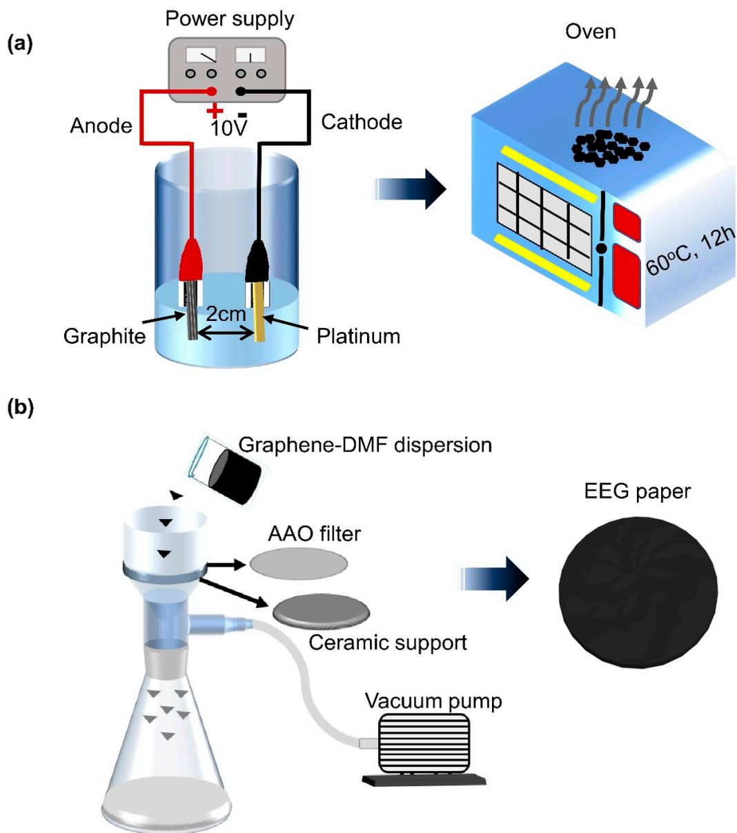
**Figure S1.** Schematic illustration of the fabrication of the EEG paper: (a) Electrochemical exfoliation of graphite. (b) Preparation of the EEG paper using vacuum filtration.
