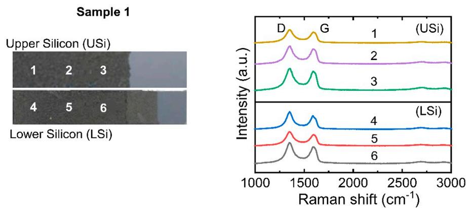
**Figure S6.** Raman spectra of the EEG paper after fracture.
