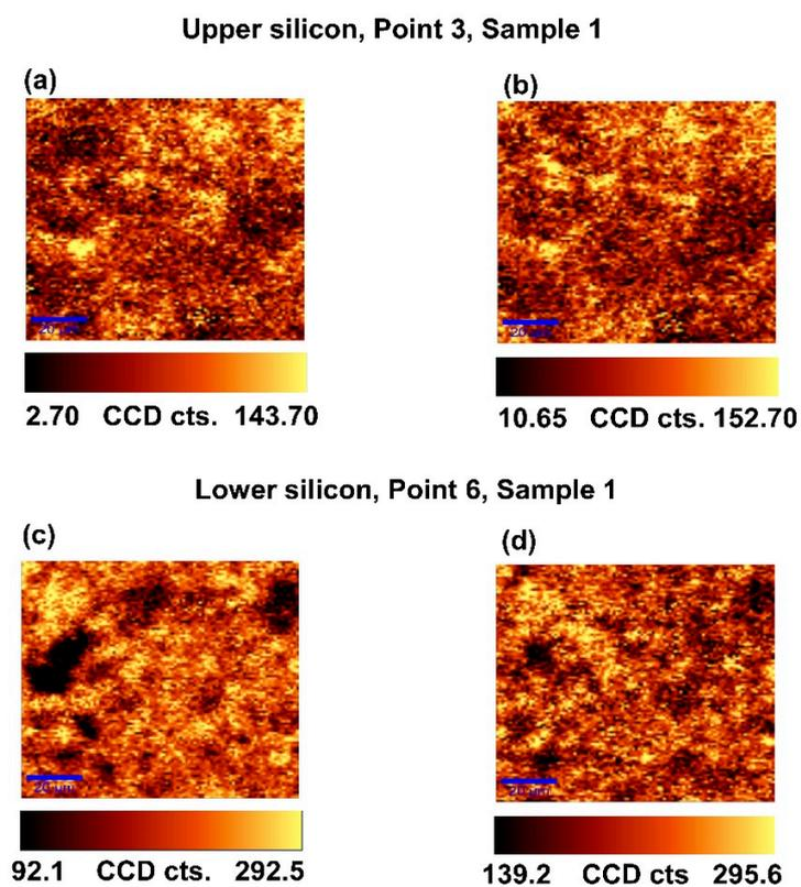
**Figure S7.** Raman intensity maps of (a, c) the D band and (b, d) the G band for the fracture surface. The fractured EEG paper was positioned at point 3 and point 6 indicated in Figure S6. The mapping area was  $100 \times 100 \mu\text{m}$ . Scale bar =  $20 \mu\text{m}$ .
