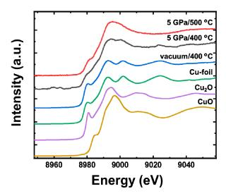
Figure 4. XANES spectra of MOF-derived Cu@C and reference samples.
