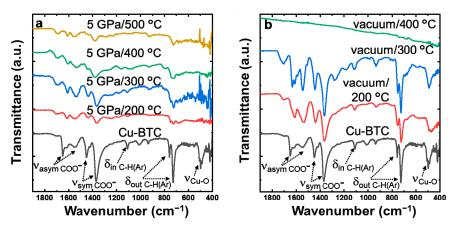
**Figure 2.** FTIR spectra of (**a**) the HPHT samples and (**b**) the samples pyrolyzed in the vacuum-sealed glass tubes. Marks of IR peaks v,  $\delta$ , and Ar in the figures denote stretching, bending, and the benzene ring, respectively.
