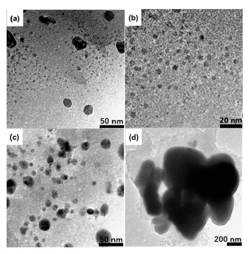
**Figure 3.** TEM images of (**a**) Cu@C synthesized at 5 GPa/500 °C, (**b**) magnified view of (**a**), (**c**) Cu@C synthesized at 5 GPa/400 °C, and (**d**) Cu@C synthesized in a vacuum-sealed glass tube (vacuum/400 °C).
