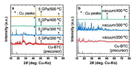
**Figure 1.** X-ray diffraction patterns of (**a**) the HPHT samples and (**b**) the samples pyrolyzed in the vacuum-sealed glass tubes. The peaks marked with an asterisk (\*) at  $2\theta = 43.4^{\circ}$ ,  $50.5^{\circ}$ , and  $74.1^{\circ}$  are assigned to (110), (200), and (220) crystalline planes of metallic Cu, respectively.
