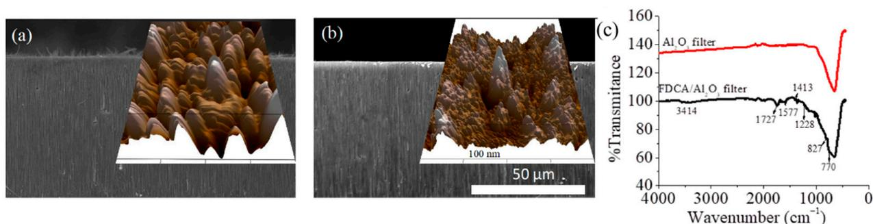
**Figure 1.** (a) SEM micrograph, cross-section of FDCA/Al<sub>2</sub>O<sub>3</sub> functionalized filter; Insert: atomic force microscope (AFM) surface roughness; (b) SEM micrograph, cross-section of Al<sub>2</sub>O<sub>3</sub> filter used as control; Insert: AFM surface roughness; (c) FTIR spectra of FDCA/Al<sub>2</sub>O<sub>3</sub> functionalized filter relative to control.
