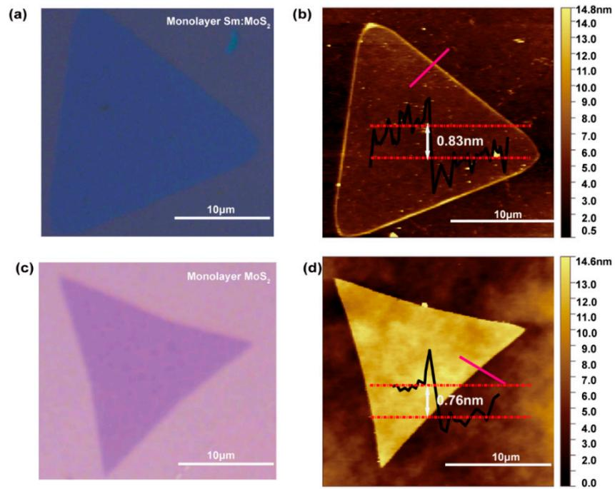
**Figure S4.** Optical microscopy images of (a) Sm-doped and (c) undoped MoS<sub>2</sub> triangles. AFM images and the height of (b) Sm-doped and (d) undoped MoS<sub>2</sub>. Scale bars: 10 μm.
