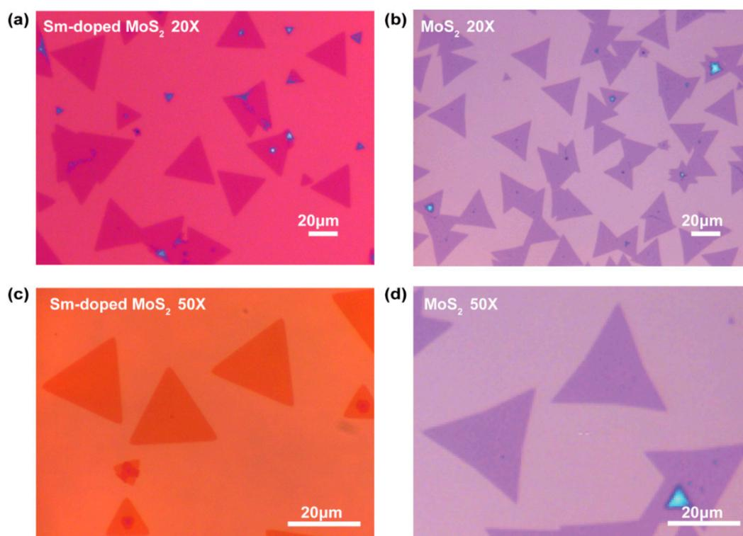
**Figure S2.** Optical image of triangular monolayer Sm-doped  $\text{MoS}_2$  (a) and triangular monolayer  $\text{MoS}_2$ (b) islands CVD-grown on  $\text{SiO}_2/\text{Si}$  substrates on a Si substrate under a 20X optical microscope. Optical image of triangular monolayer Sm-doped  $\text{MoS}_2$  (c) and triangular monolayer  $\text{MoS}_2$ (d) islands CVD-grown on  $\text{SiO}_2/\text{Si}$  substrates on a Si substrate under a 50X optical microscope.
