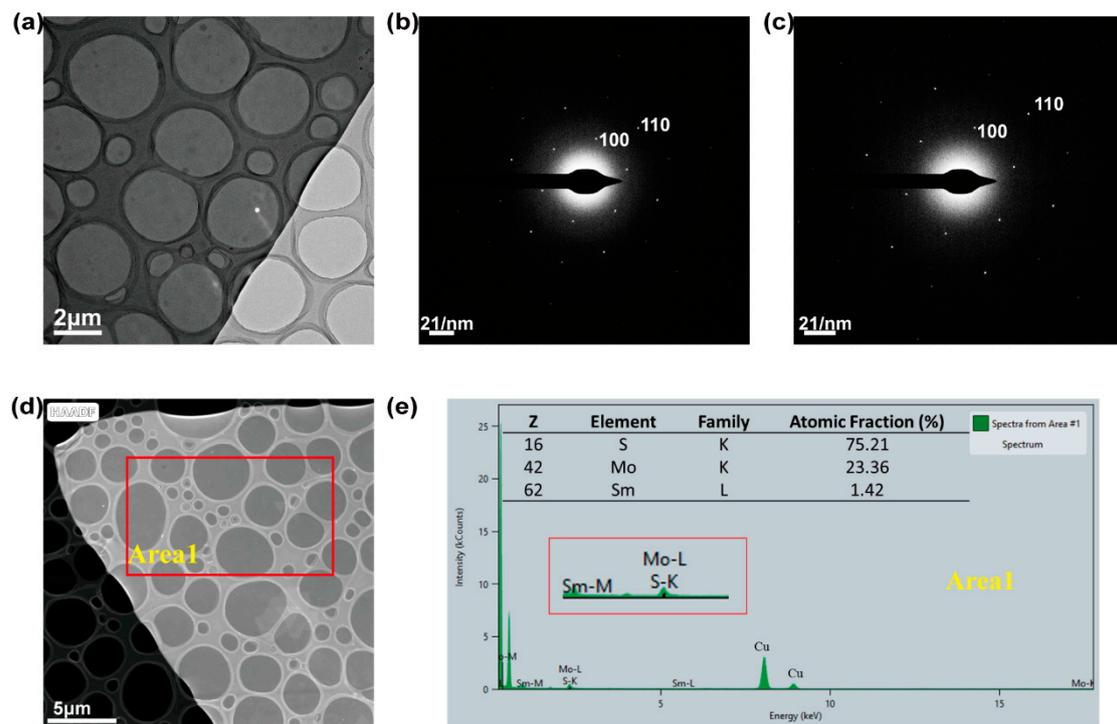
**Figure S5.** (a) Low-magnification TEM image of Sm-doped MoS<sub>2</sub> single crystal on a Cu grid. SAED patterns (b-c) collected from different sites on the monolayer triangle Sm-doped MoS<sub>2</sub>. (d) Low-magnification TEM image of Sm-doped MoS<sub>2</sub>, the red box shows the measured area of figure (e). EDS spectrum (e) of Sm-doped MoS<sub>2</sub> with Mo, Sm, and S labeled and inset showing the atomic percent of
