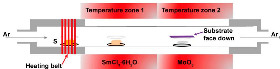
**Figure S1.** Schematic of the CVD system for growth of monolayer Sm-doped  $\text{MoS}_2$  film on  $\text{SiO}_2/\text{Si}$  substrate.
