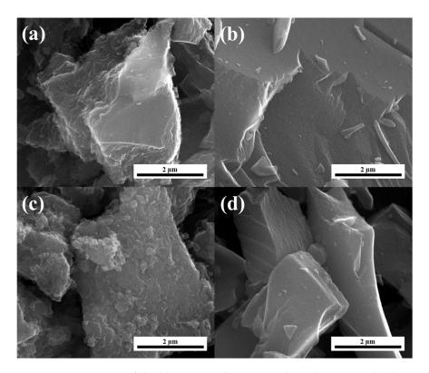
**Figure 1.** SEM images of the (a) mixture of sucrose and graphene nanoplatelets with a 3:1 ratio (SGF-3:1), (b) mixture of sucrose and chitosan with a 3:1 ratio (SCS-3:1), (c) mixture of sucrose and graphene nanoplatelets with a 5:3 ratio (SGF-5:3), and (d) mixture of sucrose and chitosan with a 5:3 ratio (SCS-5:3) sample.
