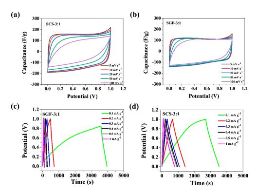
**Figure 5.** Electrochemical performance tests of the SCS-3:1 and SGF-3:1 samples:  $(\mathbf{a},\mathbf{b})$  cyclic voltammetry (CV) profiles at different scan rates ranging from 5 to 100 mV s<sup>-1</sup>;  $(\mathbf{c},\mathbf{d})$  galvanostatic charge-discharge curves.
