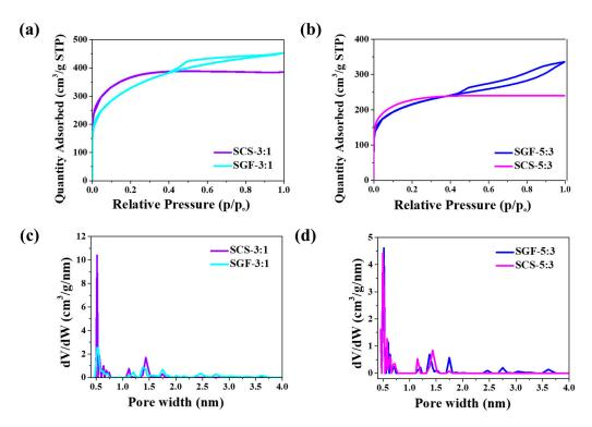
Figure 2. (a,b)  $N_2$  adsorption–desorption isotherms at 77 K; (c,d) nonlocalized density functional theory (NLDFT) pore size distribution obtained from adsorption branches of  $N_2$  in the SGF-R and SCS-R samples.
