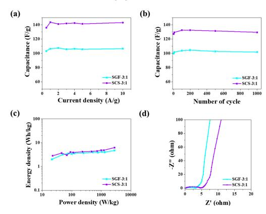
**Figure 6.** Electrochemical performance tests of the SCS-3:1 and SGF-3:1 samples: (**a**) specific capacitance as a function of current density; (**b**) specific capacitance as a function of cycle number; (**c**) specific capacitance as a function of power density; (**d**) Nyquist plot.
