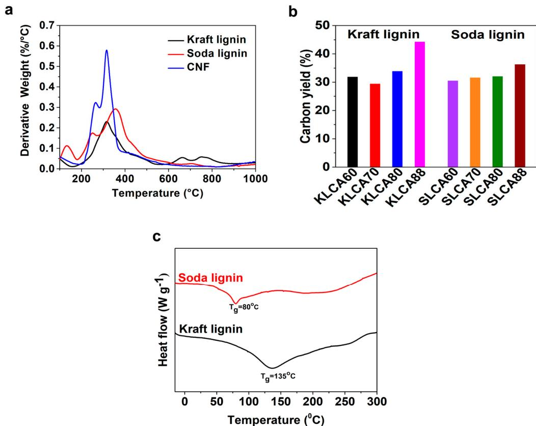
**Figure S1.** (a) Derivative thermogravimetric (DTG) curve of kraft, soda and CNF; (b) carbon yield for KL- and SL-based carbon aerogels; (c) differential scanning calorimetry (DSC) curves for kraft lignin and soda lignin.
