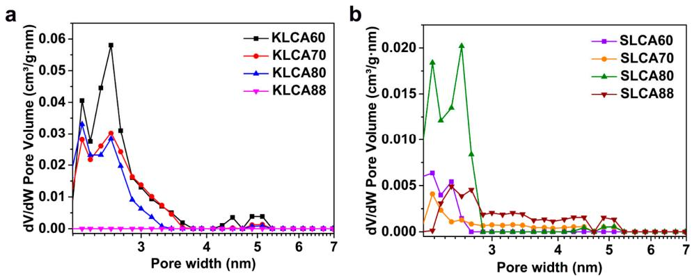
**Figure S6.** Pore size distribution of a) KLCAs and b) SLCAs (represented as differential pore volume plotted against pore width) derived from adsorption isotherms of KLCAs and SLCAs and calculated with the NLDFT model.
