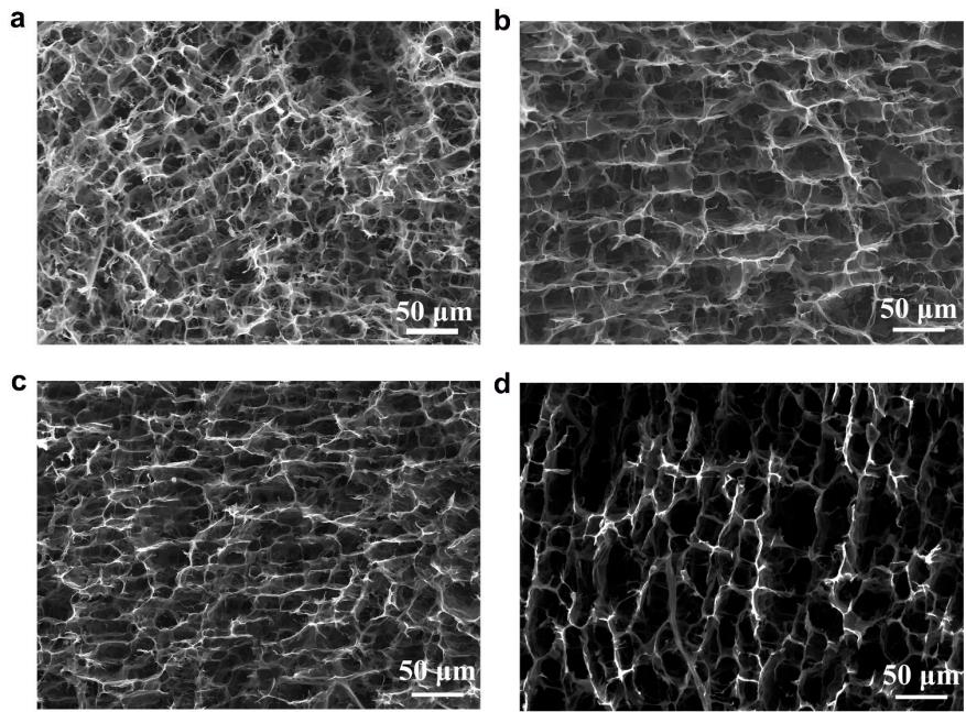
**Figure S2.** Honeycomb-like micro-structure in the cross section of CAs (a) SLCA60 (b) SLCA70 (c) SLCA80 and (d) SLCA88.
