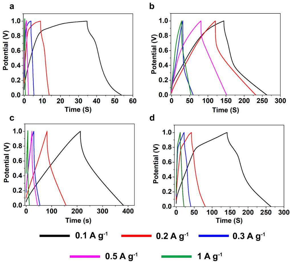
**Figure S8.** Galvanostatic charge-discharge (GCD) curves for soda lignin based carbon aerogels. (a) SLCA60 (b) SLCA70 (c) SLCA80 and (d) SLCA88.
