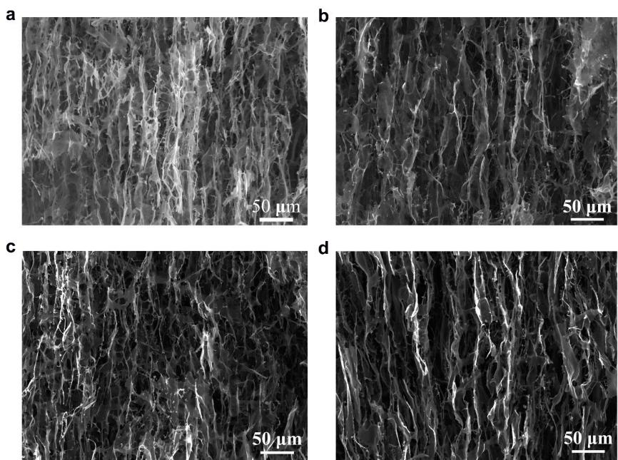
**Figure S3.** Longitudinal channel like micro-structure in the CAs (a) SLCA60 (b) SLCA70 (c) SLCA80 and (d) SLCA88.
