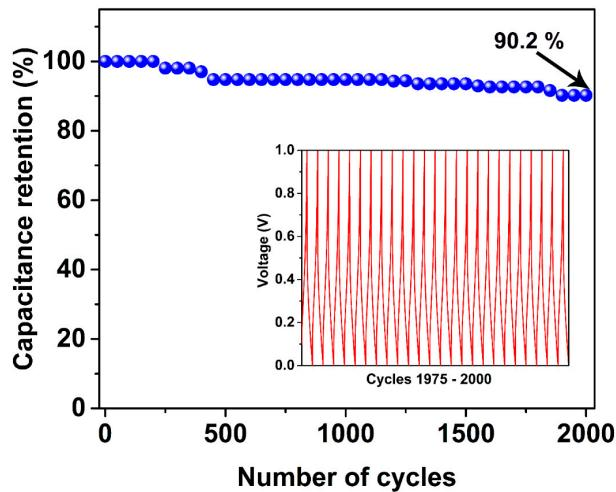
**Figure S9.** Cyclic stability of KLCA60 electrodes after 2000 charge-discharge cycles.
