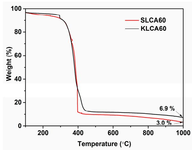
**Figure S4.** Thermogravimetric analysis of SLCA60 and KLCA60 in oxygen atmosphere.
