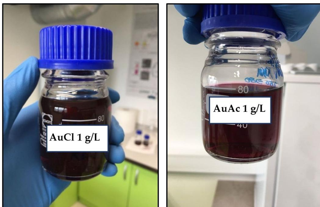
**Figure 2.** Prepared gold inks gold (III) chloride tetrahydrate (AuCl) and Au acetate salt (AuAc) with Au concentration of 1 g/L in the precursor.
