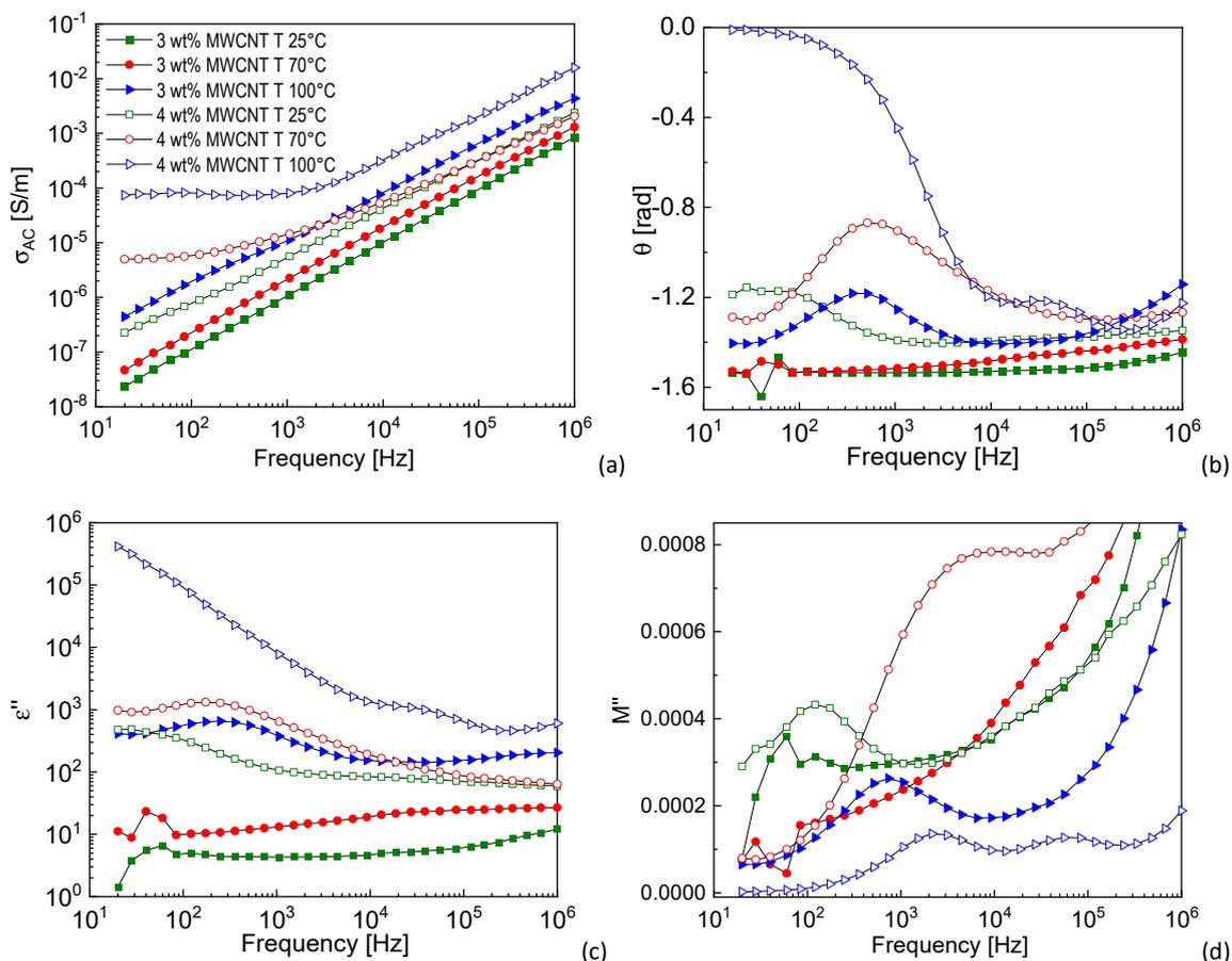
**Figure 3.** (a)  $\sigma_{AC}$ , (b) phase angle, (c)  $\epsilon''$  and (d)  $M''$  of 3 and 4 wt%-multi-walled carbon nanotube (MWCNT) nanocomposites manufactured at temperature of the mold 25-70-100 °C (tests executed in P1; graph legend reported in (a) is valid for all the graphs).
