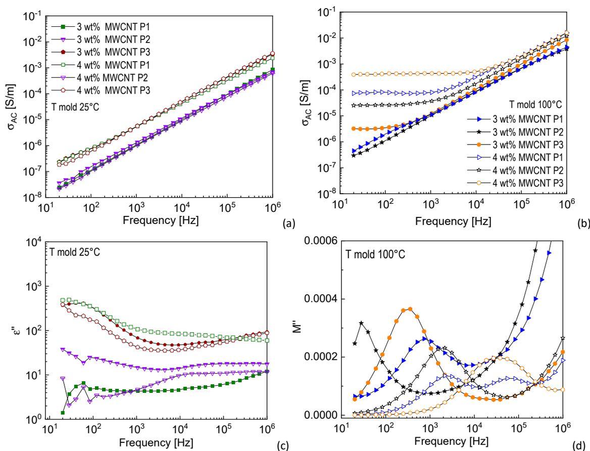
**Figure 4.** (a,b)  $\sigma_{AC}$  curves of 3 and 4 wt%-MWCNT nanocomposites manufactured at mold temperatures (a) 25 °C and (b) 100 °C. (c,d)  $M''$  curves of 3 and 4 wt%-MWCNT nanocomposites manufactured at mold temperatures (c) 25 °C and (d) 100 °C (graph legend reported in (a) is valid also for (c); graph legend reported in (b) is valid also for (d)).
