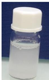
Figure S18. Monoclinic KLuW nanocrystals dispersed in distilled water.
