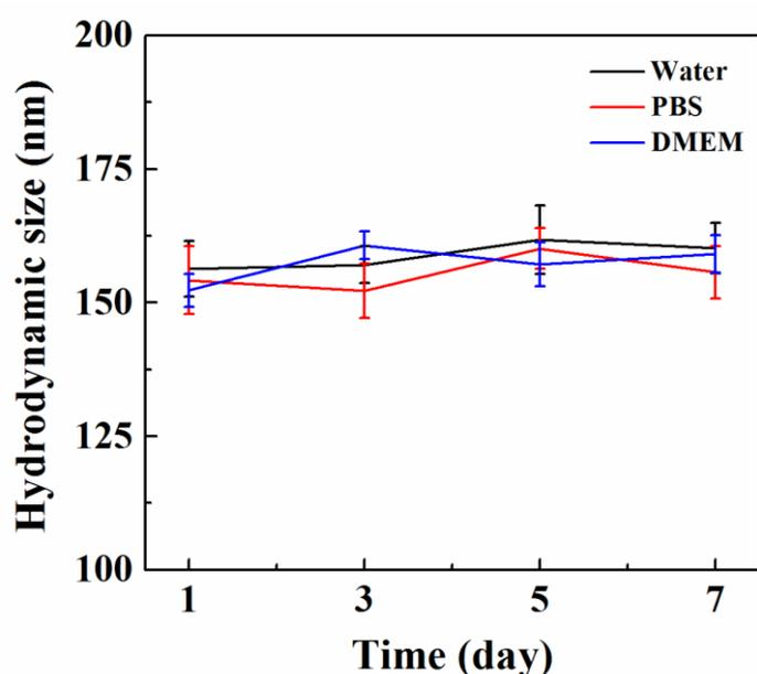
**Figure S1.** Hydrodynamic size of ICG/LAP-PDA-PEG-RGD/DOX dispersed in water, PBS and DMEM in 7 days.
