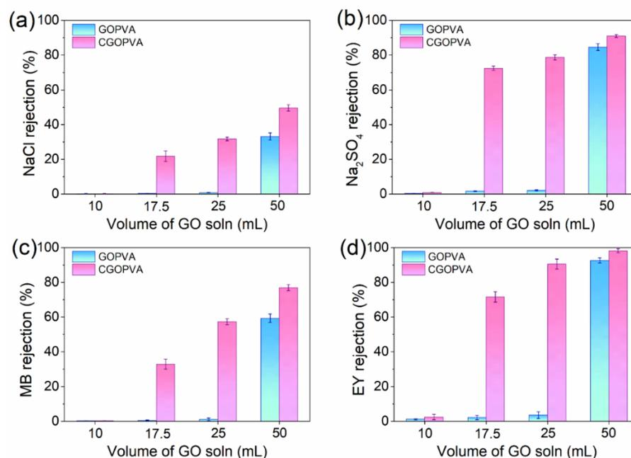
**Figure 7.** Rejection performances of GOPVA and CGOPVA membranes for (a) NaCl 20 mM, (b) Na<sub>2</sub>SO<sub>4</sub> 20 mM, (c) MB 10 mg/L, and (d) EY 10 mg/L in terms of filtration volume of GO and GO-GA solutions (10, 17.5, 25, and 50 mL), applied pressure = 5 bar and cross-flow velocity = 8.3 cm<sup>-1</sup>.
