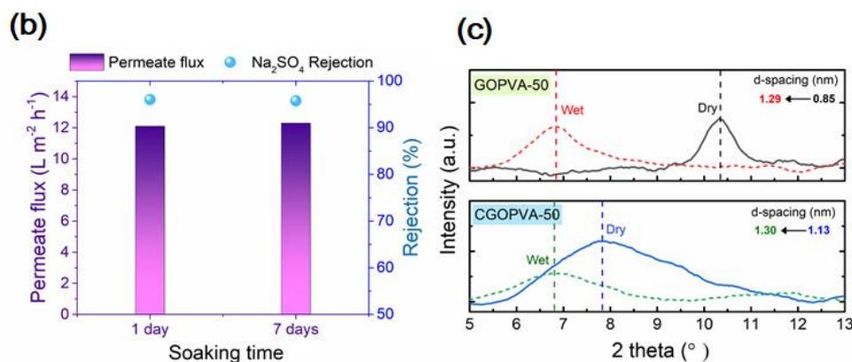
**Figure 9.** (a) Physical stability of GO-PVA composite membranes via ultrasonication method. (b) Membrane performance of CGOPVA-50 membrane as a function of soaking time in DI water (feed solution: Na<sub>2</sub>SO<sub>4</sub> 10 mM, applied pressure: 5 bar, and cross-flow velocity: 8.3 cm<sup>-1</sup>). (c) XRD spectra and d-spacings of GOPVA-50 and CGOPVA-50 membranes at dry and wet states.
