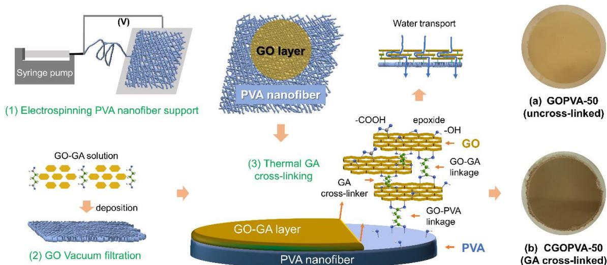
**Figure 1.** Schematic illustration for the preparation of the cross-linked GO-PVA composite membrane (CGOPVA-50) by GA cross-linker.
