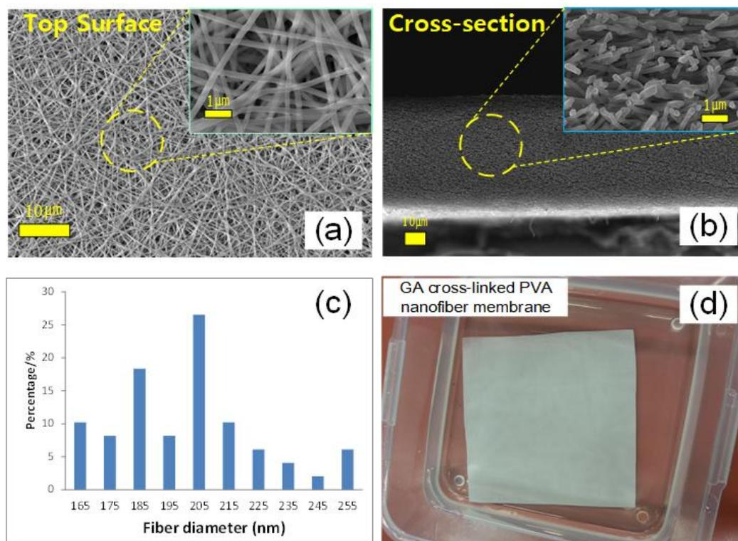
**Figure 2.** PVA nanofiber membrane prepared via electrospinning and then cross-linked via GA: SEM images of (a) top surface and (b) cross-section; (c) average nanofiber diameters from histogram; (d) water-insoluble PVA nanofiber membrane cross-linked via GA (CPVA).
