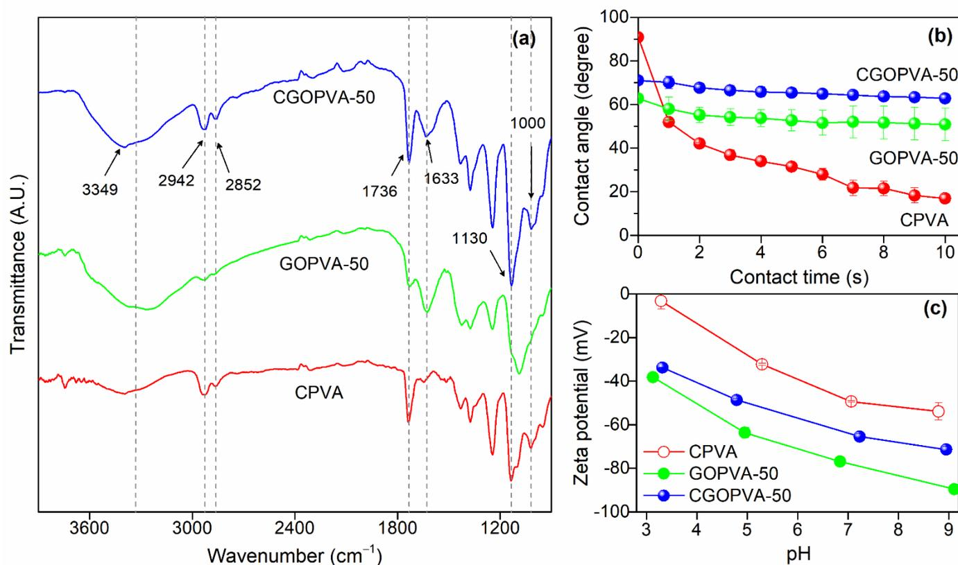
**Figure 5.** Characterization results of pure and GO-modified PVA nanofiber membranes: (a) FTIR; (b) contact angle; (c) zeta potential measurements.
