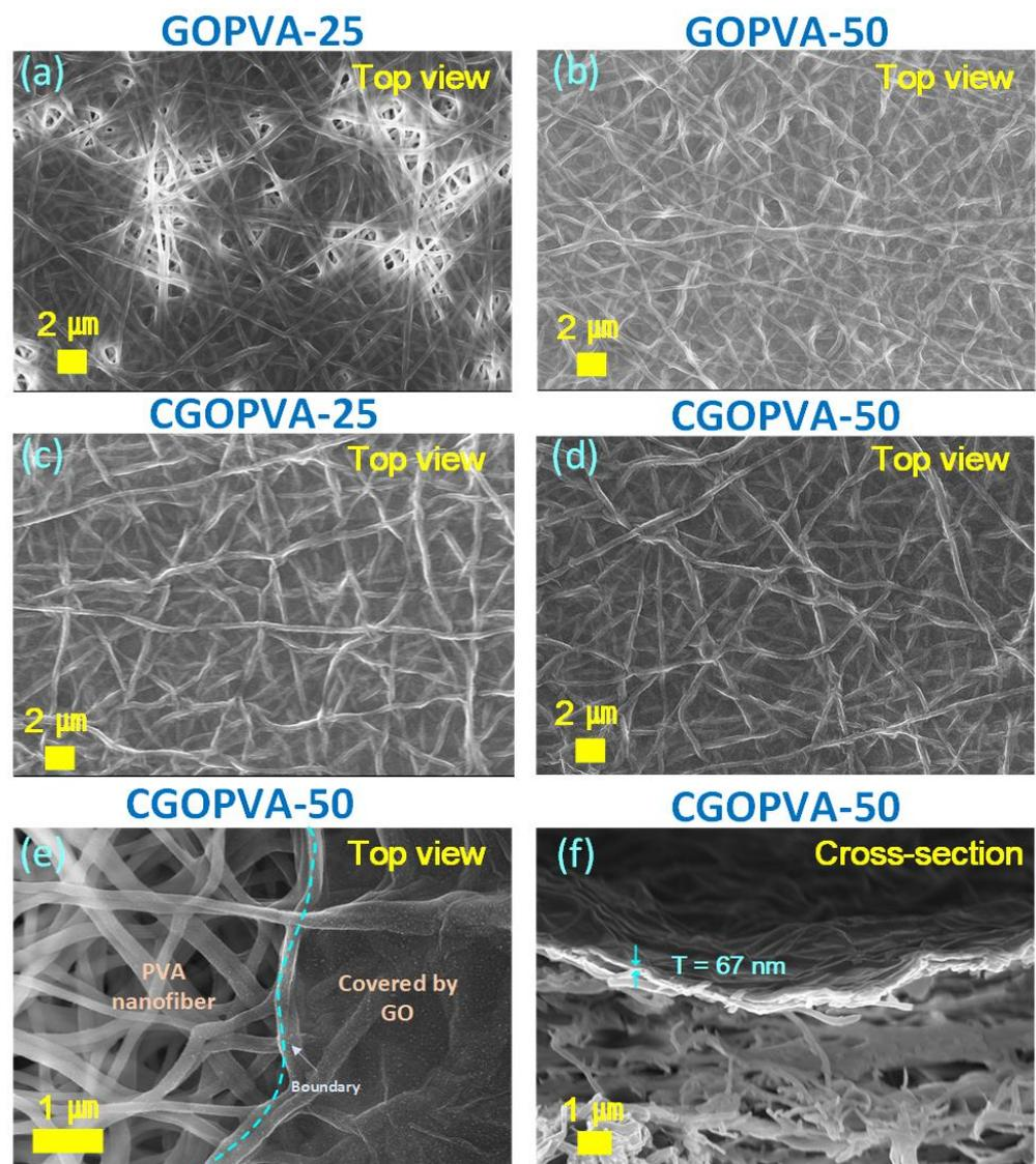
**Figure 4.** FESEM images of top view for (a) GOPVA-25, (b) GOPVA-50, (c) CGOPVA-25, and (d,e) CGOPVA-50 and of cross-section for (f) CGOPVA-50.
