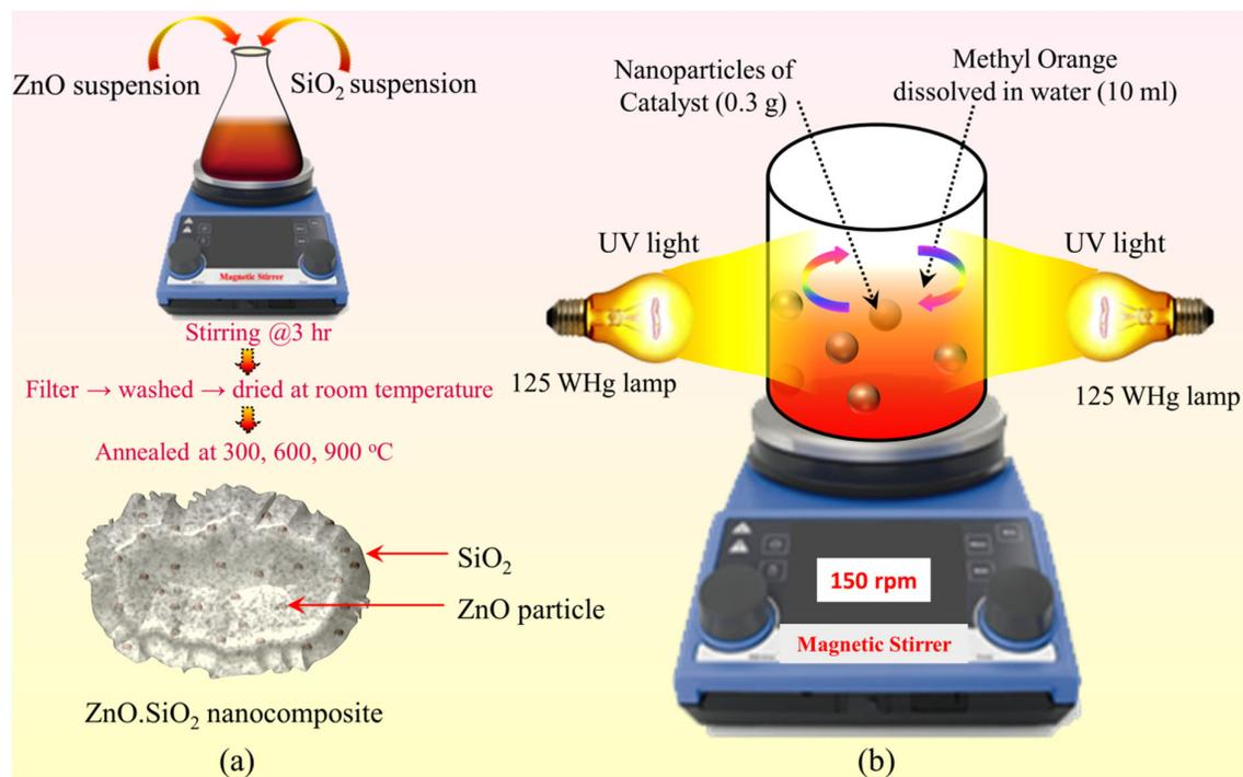
**Scheme 1.** Schematic diagram of (a) preparation of SiO<sub>2</sub>.ZnO nanoparticles with the expected morphology (ZnO nanoparticles embedded into SiO<sub>2</sub> porous structure) and, (b) photocatalytic activity set-up.
