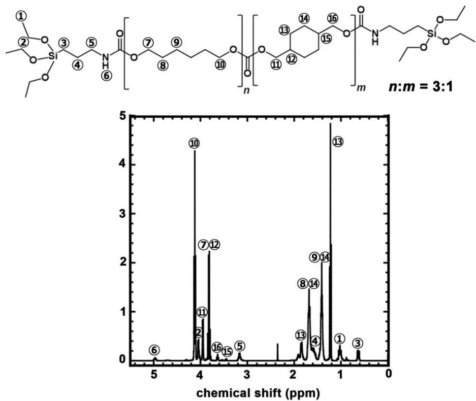
Figure S2.  $^1\text{H}$ -NMR spectrum of ET-coPCD 31.
