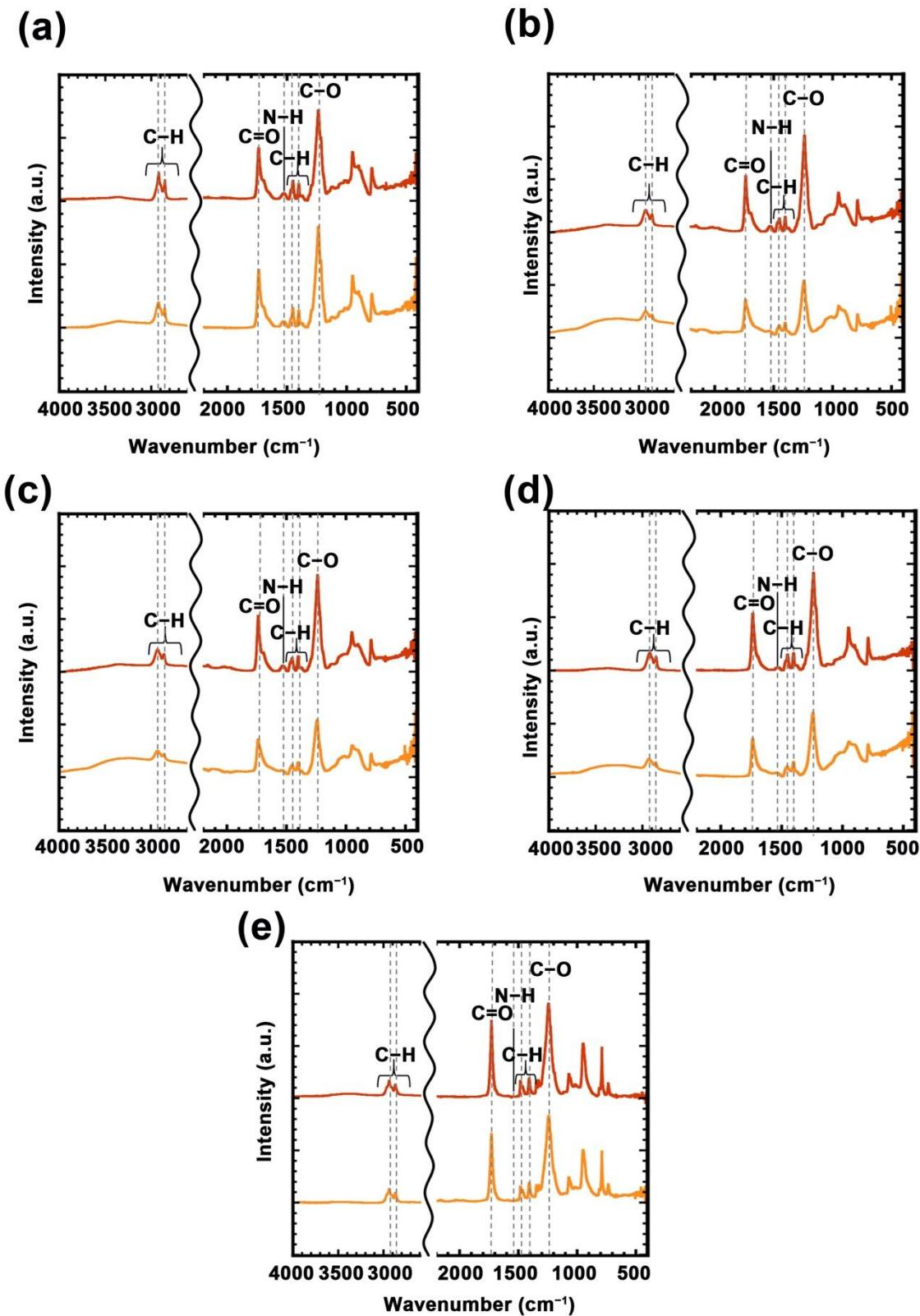
**Figure S8.** FT-IR spectral profiles of hybrid films: before UV irradiation (red line), UV irradiation after 12 h (orange line), (a) PC100, (b) PC75, (c) PC50, (d) PC25, and (e) PC0.
