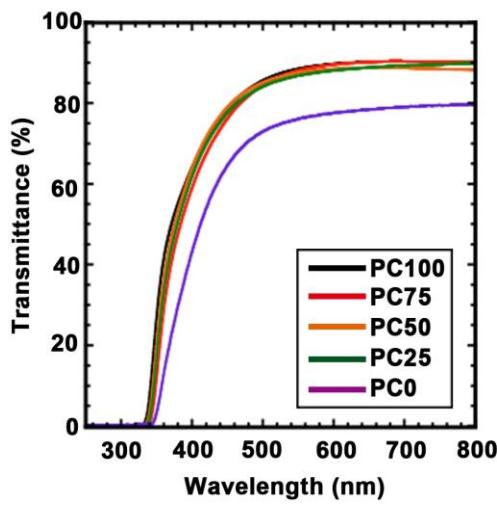
**Figure S6.** UV-Vis spectra of different hybrid films 10 days after UV irradiation: PC100 (black), PC75 (red), PC50 (orange), PC25 (green), and PC0 (purple).
