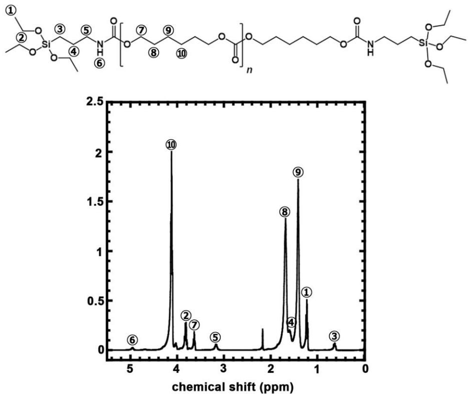
**Figure S1.** <sup>1</sup>H-NMR spectrum of ET-PHMCD.
