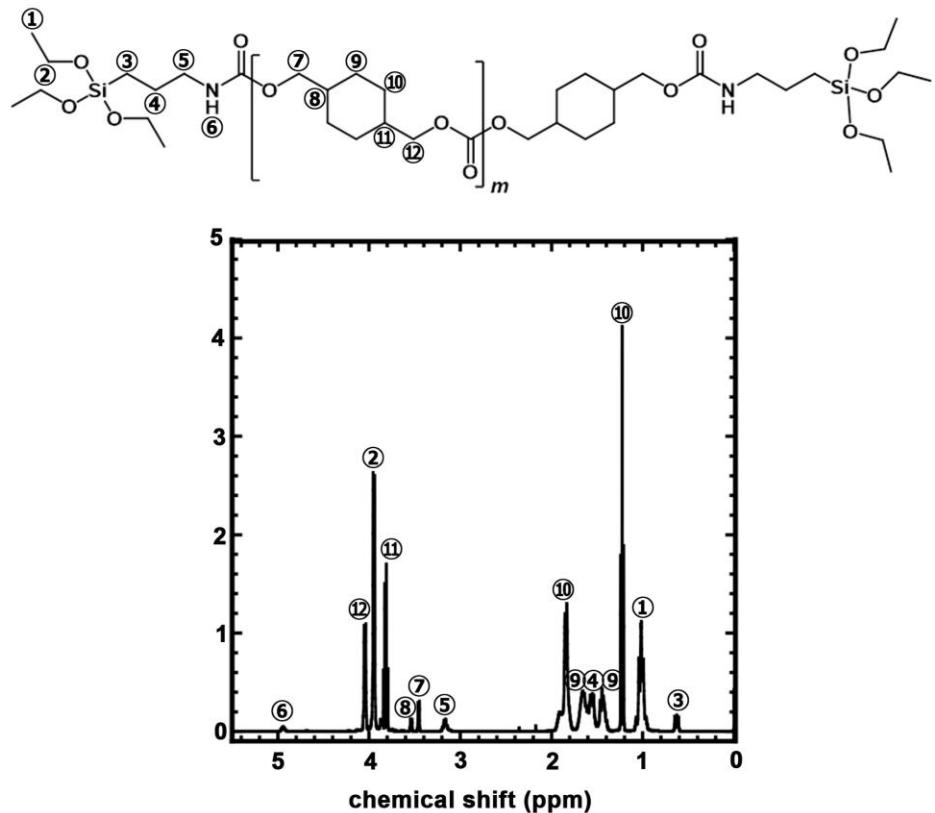
Figure S5. <sup>1</sup>H-NMR spectrum of ET-PCHCD.
