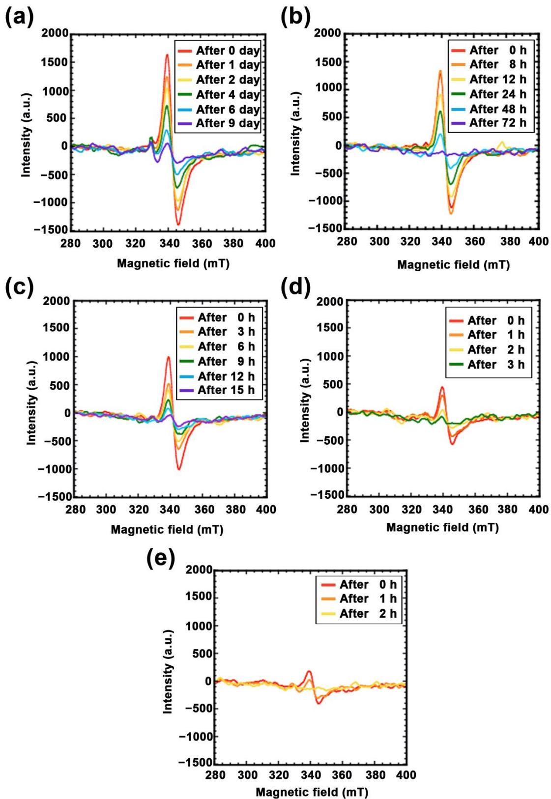
**Figure S9.** ESR spectral profiles of hybrid films after UV irradiation: (a) PC100, (b) PC75, (c) PC50, (d) PC25, and (e) PC0.
