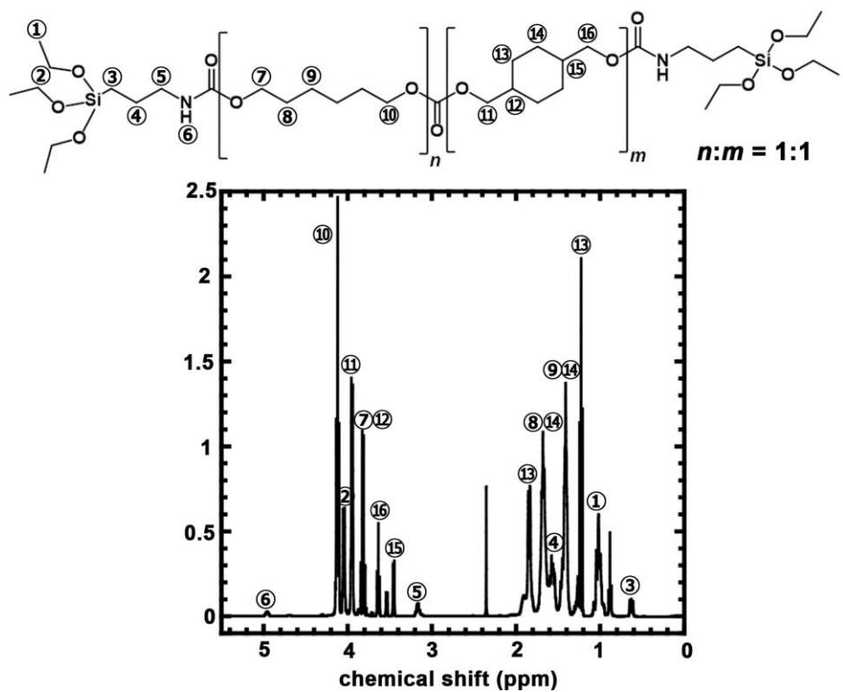
Figure S3.  $^1\text{H}$ -NMR spectrum of ET-coPCD 11.
