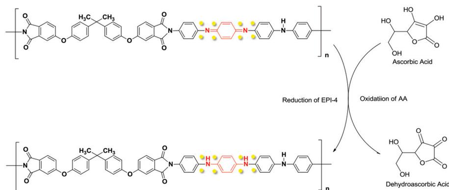
**Figure 15.** Scheme of EPI-4 structure used into a CPE to determinate AA. Yellow points represent gold nanoparticles. Reproduced with permission from [155]. Copyright 2017 Elsevier.
