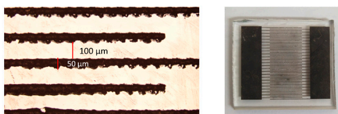
Figure S1. Microscopic and camera image of screen-printed interdigitated electrodes.
