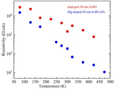
Figure S1: Resistivity of the 50 nm thick undoped and Mg-doped h-BN (sample D) versus temperature.
