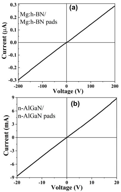
Figure S3: (a), (b): I-V characteristics measured on two Mg doped BN contact pads and two n-AlGaN contact pads.
