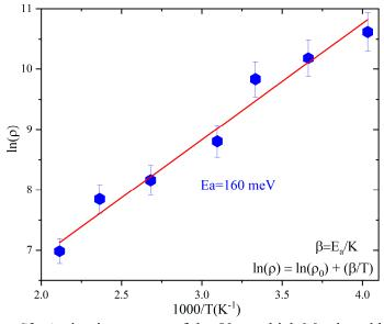
Figure S2: Activation energy of the 50 nm thick Mg-doped h-BN.
