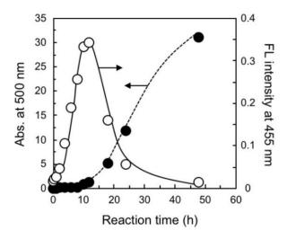
**Figure 3.** Time courses of the absorbance increase (solid circles) at 500 nm and the fluorescence change (open circles) at 455 nm upon excitation at 400 nm in the polymerization of DHN with TMTA. The polymerization condition is summarized in  $P_h$ -1 of Table 1.
