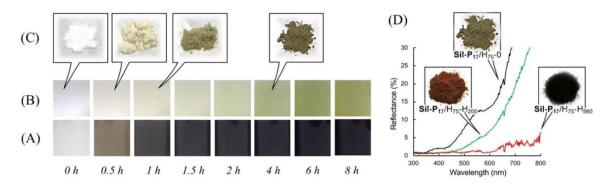
**Figure 4.** Monitoring of the color change during the polymer lamination process. The polymerization was carried out using 1 g of **Sil-0**, 120 mg of DHN, and 97 mg of TMTA in ethanol at 75 °C. (**A**) and (**B**) show the color difference of the sample suspensions without dilution and with dilution to 1/10, respectively. (**C**) shows the color difference of the corrected solid. (**D**) shows the reflection spectra of the corrected solid.
