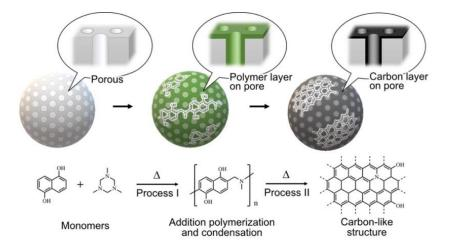
**Figure 1.** Schematic illustration of black layer-laminated porous silica through bottom-up carbon structure creation from 1,5-dihydroxynaphthalene (DHN) and 1,3,5-trimethyl-1,3,5-triazinane (TMTA), and its estimated reaction mechanism.
