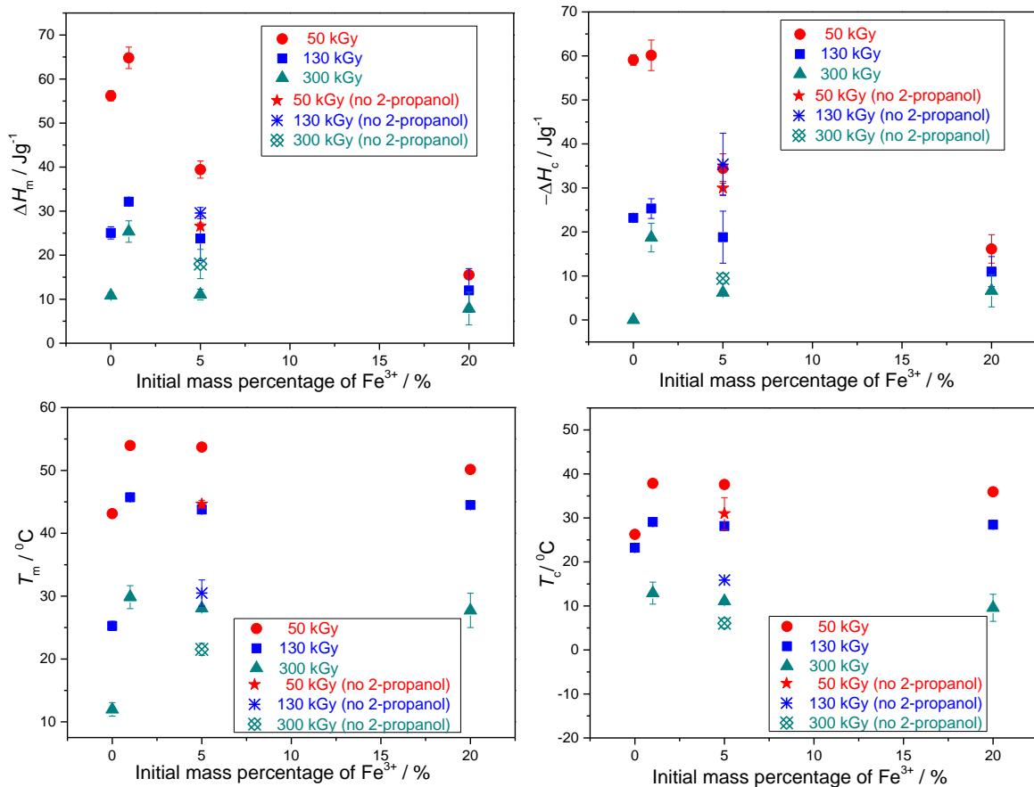
**Figure S4.** Melting ( $\Delta H_m$ ) and crystallization ( $\Delta H_m$ ) enthalpies and temperatures ( $T_m$  and  $T_c$ ) of the 2<sup>nd</sup> heating cycles and the 1<sup>st</sup> cooling cycles, respectively, of gels obtained at various doses in dependence on the mass percentage of  $Fe^{3+}$  in 1.85 wt% PEO precursor suspensions. Unless otherwise indicated suspensions contained 0.2 M 2-propanol.
