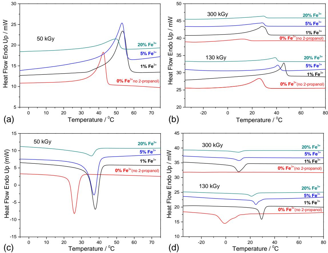
**Figure S2.** DSC thermographs of the 2<sup>nd</sup> heating (a,b) and the 1<sup>st</sup> cooling (c,d) cycles of pure PEO gel and nanocomposite gels obtained at 50, 130 and 300 kGy from 1.85 wt% PEO precursor suspensions with various Fe<sup>3+</sup> content. Unless otherwise indicated, suspensions contained 0.2 M 2-propanol.
