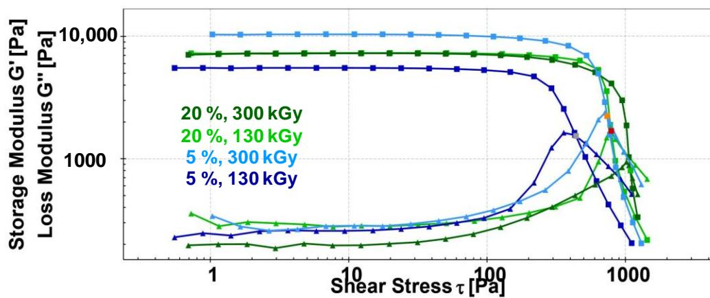
**Figure S5.** Comparison of amplitude sweep test ( $G'$  (■) and  $G''$  (▲) values) of nanocomposite gels obtained at 130 kGy and 300 kGy (1.85 wt% PEO solution), at 25°C. Initial mass percentage of  $Fe^{3+}$  in precursor suspensions is indicated.
