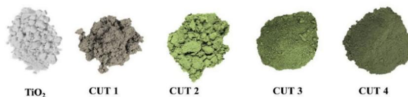
**Figure 5.** Colour of synthesized pristine and Cu-TiO<sub>2</sub>/CuO composite nanopowders. This figure is reprinted from [62], with permission from Elsevier, 2020.
