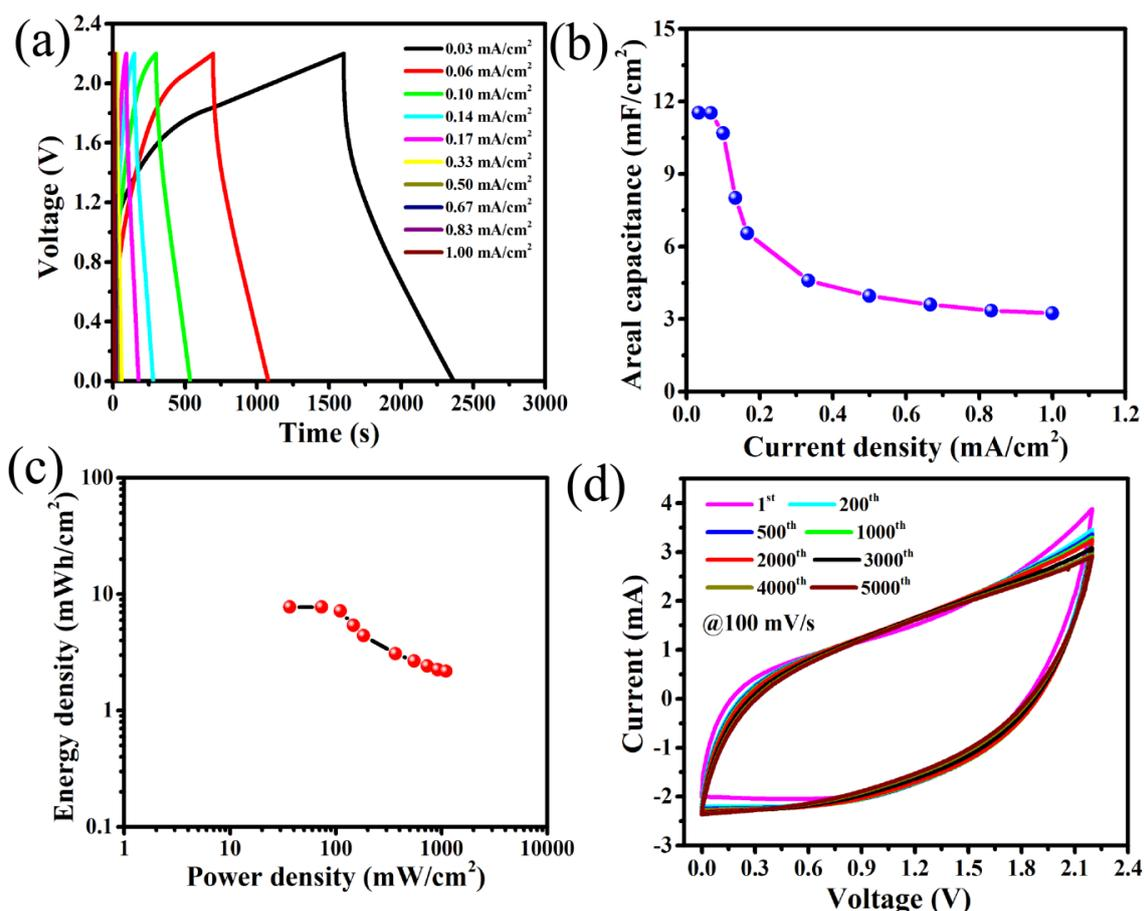
**Figure 3.** (a) Galvanostatic charge–discharge (GCD) at different current densities, (b) areal capacitance vs. current density, (c) Ragone plot and (d) 5000 CV measurements of Mn/MnO<sub>x</sub>@Graphite electrodes based FSC.
