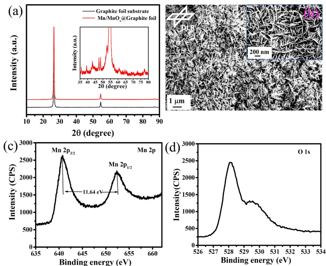
**Figure 1.** (a) XRD patterns, (b) FE-SEM images, (c,d) XPS spectra of Mn 2p and O 1s of Mn/MnO<sub>x</sub>@Graphite-foil electrode.
