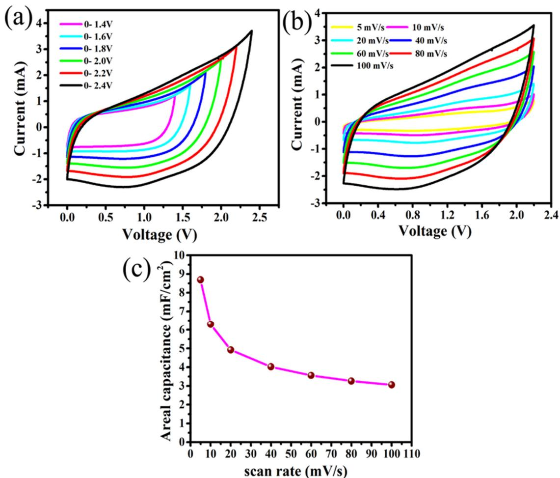
**Figure 2.** (a) Cyclic-voltammetry (CV) at different potential windows, (b) CV at different scan rate and (c) areal capacitance vs. scan rate of flexible supercapacitor (FSC) based on Mn/MnO<sub>x</sub>@Graphite-foil electrodes and polymer gel electrolyte.
