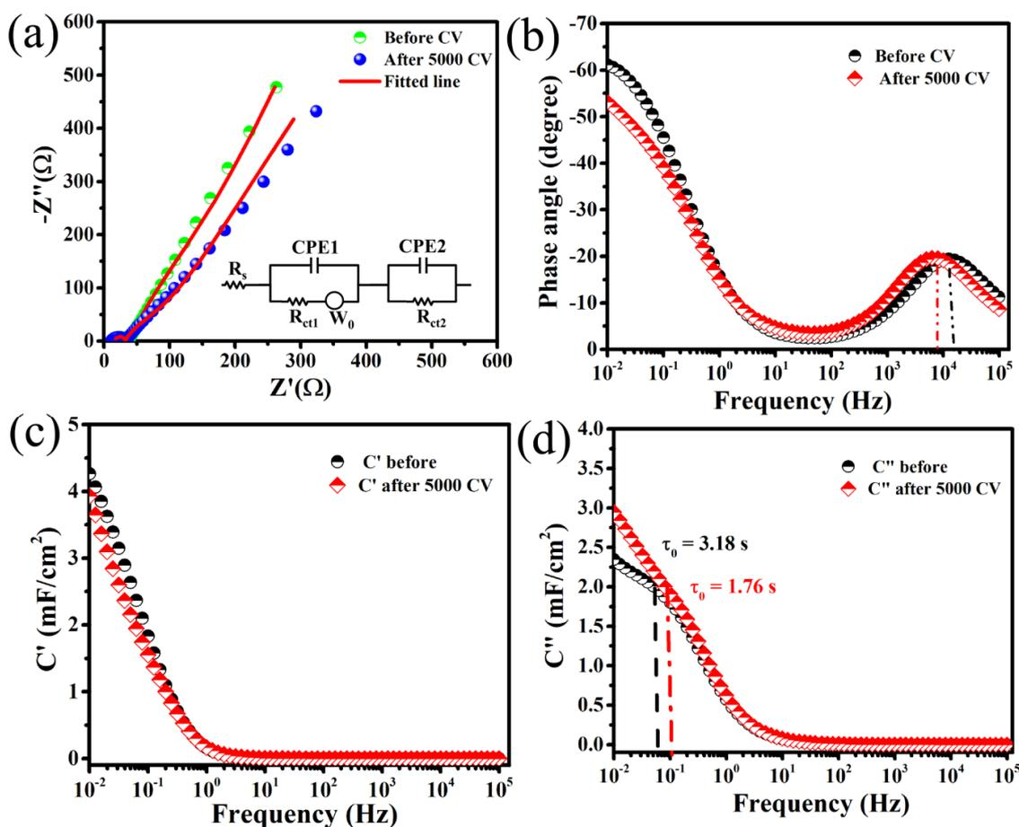
**Figure 4.** (a) Electrochemical impedance spectroscopy (EIS) before and after 5000 cycles with equivalent circuit (inset), (b) Bode plots, (c) Real part of capacitance ( $C'$ ) vs. frequency and (d) Imaginary part of capacitance ( $C''$ ) vs. frequency of FSC based on polymer electrolyte gel and Mn/MnO<sub>x</sub>@Graphite-foil electrodes.
