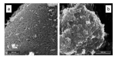
Figure 1. FEG-SEM images of (a) 2Co\_MnO2 and (b) 2Fe\_MnO2.
