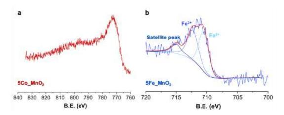
**Figure S2.** XP spectra of (a) Co 2p and (b) Fe 2p regions relative to 5Co\_MnO<sub>2</sub> and 5Fe\_MnO<sub>2</sub> respectively. The Co 2p region was not fitted since it falls within the same range of Mn 2s. Besides, the Fe high-resolution spectrum was deconvoluted into three peaks ascribable to Fe<sup>2+</sup>, Fe<sup>3+</sup> species and a satellite one, according to Biesinger *et al.* [65].
