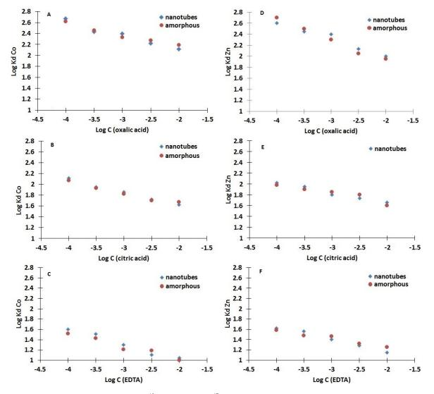
**Figure 5.** The dependence of <sup>60</sup>Co (A-C) and <sup>65</sup>Zn (D-F) cation distribution coefficients on the concentration of chelating agents
