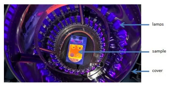
Figure 1. The interior of a photoreactor constructed by our team.
