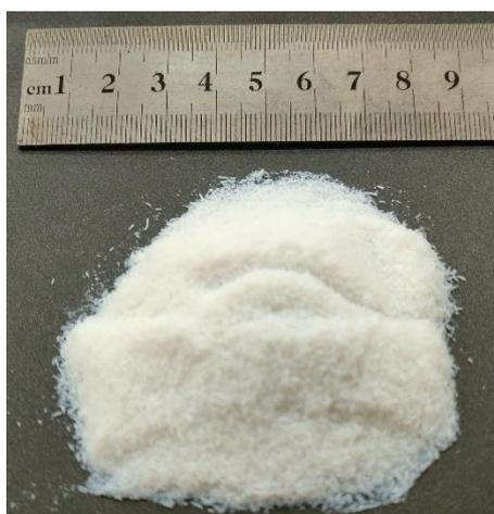
Figure S1. The synthesized Y<sub>2</sub>O<sub>3</sub>:Er<sup>3+</sup>/Tm<sup>3+</sup> UCNPs.
