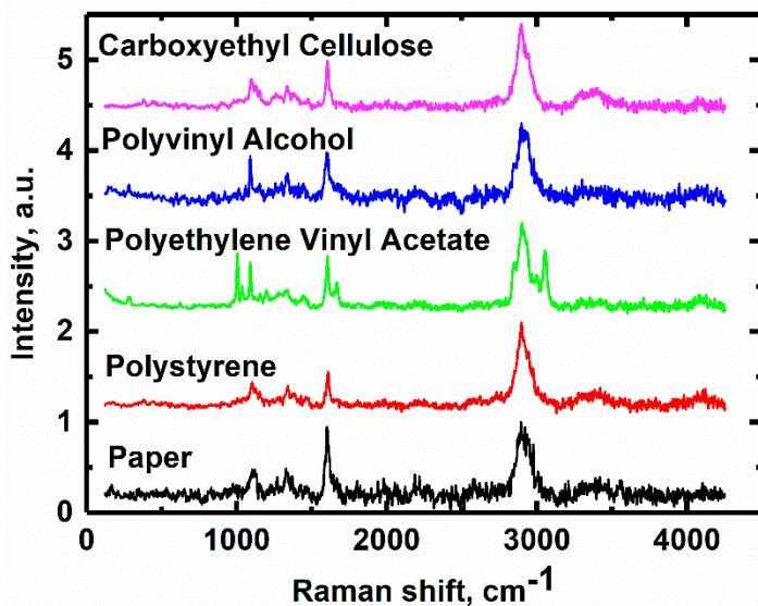
**Figure S2.** Raman spectra of the paper samples treated with a pre-coating blends.
