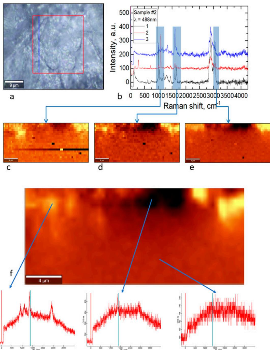
**Figure S5.** Raman spectra into the depth of the sample. a) Optical image, Raman spectra in the different points, c-e) Raman cross sections into the depth of the samples by different peaks, f) Raman spectra examples at the different depth for 1435 cm<sup>-1</sup> line.
