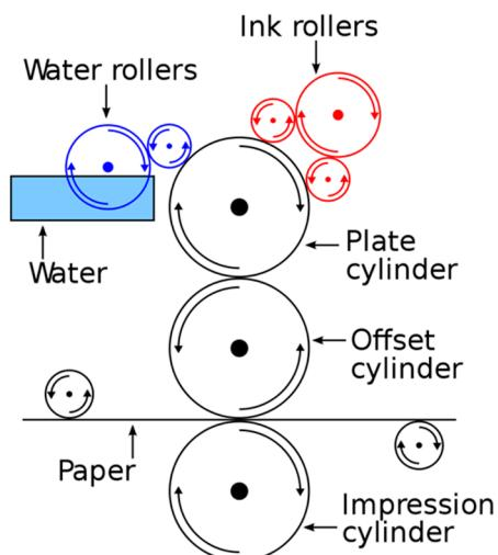
**Figure S1.** General scheme of commercial rotary printing press for offset printing.
