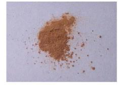
Final silicon oxide nanopowder obtained after oxidation of nanosilicon in water
