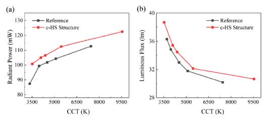
**Figure 9.** (a) Radiant power and (b) luminous flux of the reference structure and c-HS structure at different correlated color temperature (CCT) values [65]. Figure reproduced with permission from Optical Society of America.
