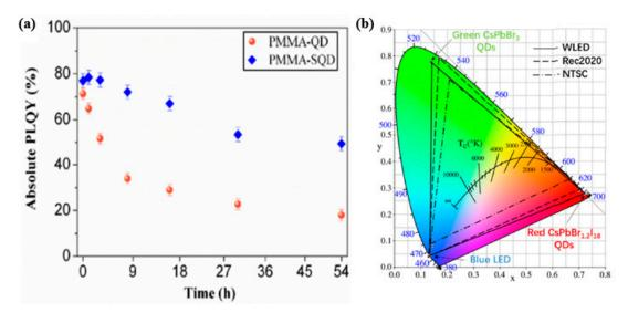
**Figure 17.** (**a**) The PLQY values under UV irradiation; (**b**) color gamut of the resulting WLED [82]. Figure reproduced with permission from Optical Society of America.
