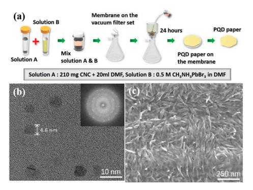
**Figure 13.** (a) Schematic of fabrication process of PQD paper. (b) TEM image of CH<sub>3</sub>NH<sub>3</sub>PbBr<sub>3</sub> PQDs. (c) SEM of PQD paper surface [78]. Figure reproduced with permission from John Wiley and Sons.
