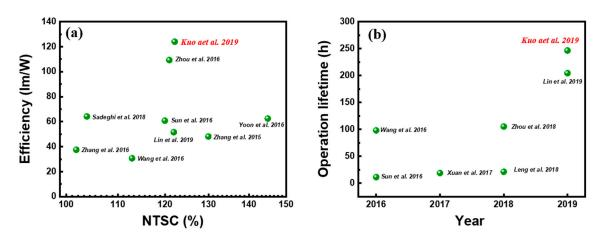
**Figure 15.** Comparison of device performance between PQD paper-based LED and other reported LEDs using QDs as color converters. (**a**) Luminous efficiency and color gamut performance and (**b**) operational durability of reported QD-based LEDs [78]. Figure reproduced with permission from John Wiley and Sons.
