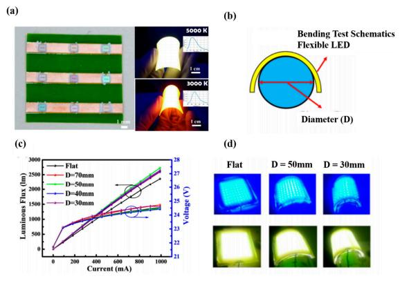
**Figure 18.** (a) LED array under optical microscope (left), phosphor layers at 5000 K and 3000 K (right top and bottom, respectively). (b) Schematic of flexible device. (c) Voltage and luminous flux with respect to current at different bending diameters for the flexible white LED. (d) Top and bottom photographs depict before and after bonding the adhesive phosphor film and blue LED arrays, respectively [85]. Figure reproduced with permission from Optical Society of America.
