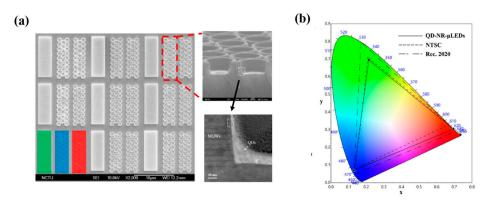
**Figure 2.** (a) Scanning electron microscopy (SEM) image of red, green, and blue (RGB) pixel array and NR-µLED with 30° tilt angle; transmission electron microscopy (TEM) image of the contact area between multi quantum wells (MQWs) and QDs. (b) Color gamut of RGB hybrid QD-NR-µLEDs, NTSC, and Rec. 2020 [46]. Figure reproduced with permission from Optical Society of America.
