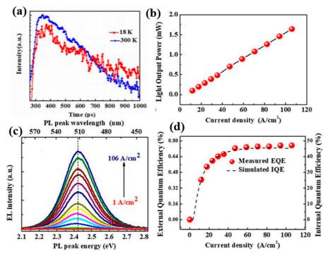
**Figure 10.** (a) TRPL measurements of capped QDs; (b) LOP versus injection current density; (c) electroluminescence spectra of QD LED; (d) EQE as a function of current density [73]. Figure reproduced with permission from Optical Society of America.
