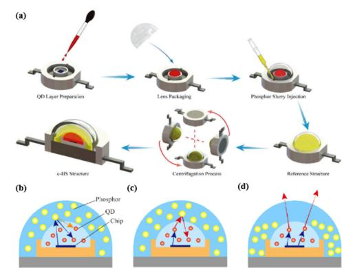
**Figure 8.** (a) Diagram of the fabrication process of WLEDs c-HS structure. Diagram of the light-extraction mechanism in Q–P hybrid WLEDs. (b) Backscattered blue light and backward-emission yellow light in the top region of reference structure; (c) backscattered red light in the top region of reference structure; (d) extraction red light with less backscattering in the top region of the c-HS structure [65]. Figure reproduced with permission from Optical Society of America.
