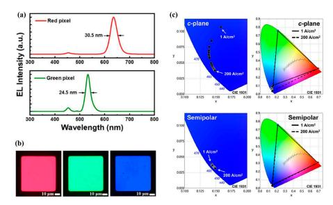
**Figure 5.** (a) EL spectra of red and green pixels. (b) EL image of RGB pixels. (c) Color gamut of RGB pixel assembly from c-plane μLED and QDPR at various current densities in CIE 1931 color space [49]. Figure reproduced with permission from Optical Society of America.
