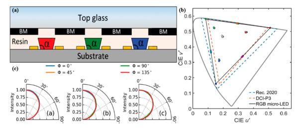
**Figure 7.** (a) RGB  $\mu$ LED display with top black matrix. (b) Simulated color shifts of ten reference colors at viewing angles from 0° to 80° for the RGB  $\mu$ LED display with a top black matrix and 120° taper angle. (c) Simulated radiation patterns for RGB  $\mu$ LEDs with top black matrix [53]. Figure reproduced with permission from Optical Society of America.
