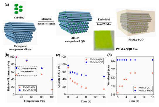
**Figure 16.** (a) A schematic diagram for the preparation process of PMMA-SQD composites; (b) the relative PL intensity as a function of heating temperature from 30 °C to 100 °C; (c) the PLQY values and (d) PL peak wavelength as a function of time when the films continuously heated at 80 °C [82]. Figure reproduced with permission from Optical Society of America.
