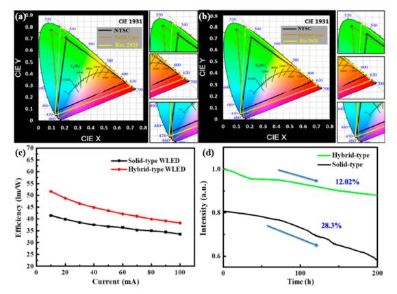
**Figure 12.** Color gamut on CIE 1931 color space for (**a**) solid and (**b**) hybrid-type WLED. (**c**) Luminance efficiency with respect to current. (**d**) Stability of solid- and hybrid-type WLEDs [74]. Figure reproduced with permission from Optical Society of America.
