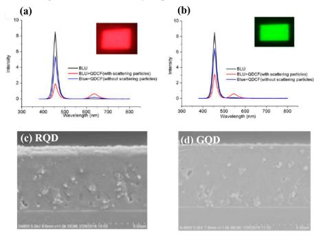
**Figure 4.** Comparison of (a) red and (b) green QDCFs spectra with and without scattering particles under blue LED backlight. (c,d) The cross-sectional SEM images of red and green QDPR on glass through photolithography process [48]. Figure reproduced with permission from John Wiley and Sons.
