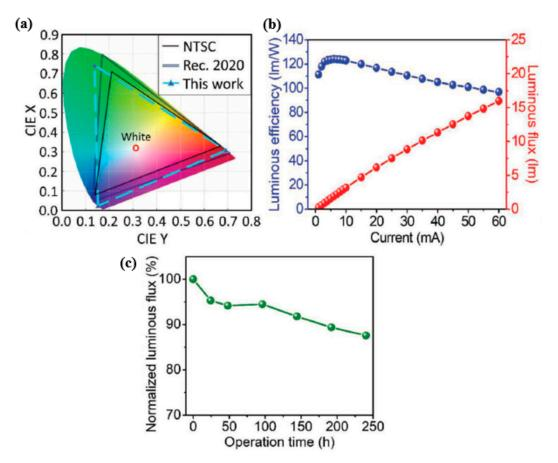
**Figure 14.** (a) CIE diagram illustrating the color gamut of the NTSC standard, the Rec. 2020 standard, and the PQD paper-based LED. (b) Current-dependent luminous efficiency and luminous flux of the PQD paper-based LED. (c) Time-dependent luminous flux of the LED device under continuous operation [78]. Figure reproduced with permission from John Wiley and Sons.
