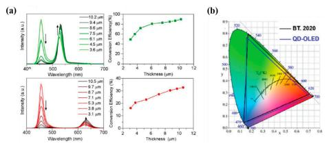
**Figure 3.** (a) Photoluminescence (PL) spectra and light conversion efficiency (LCE) of green and red QD layers at different thicknesses. (b) Color gamut of the QD-OLED display (blue triangle area), in comparison with the color gamut of BT. 2020 (black triangle area) [47]. Figure reproduced with permission from Royal Society of Chemistry.
