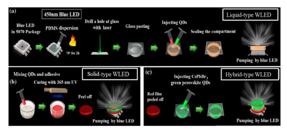
**Figure 11.** Process flow of perovskite quantum dots (PQDs)-based WLEDs: (a) liquid, (b) solid, and (c) hybrid types [74]. Figure reproduced with permission from Optical Society of America.
