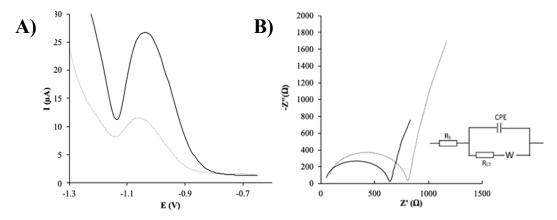
**Figure 3.** (**A**) Differential pulse anodic stripping voltammetric (DPASV) measurements of bare-SPCNFE and Ag-NS-SPCNFE sensors obtained for 50 and 25  $\mu$ g L<sup>-1</sup> of As(V) in 0.01 mol L<sup>-1</sup> HCl pH 2, respectively. (**B**) Nyquist diagram for bare-SPCNFE and Ag-NS-SPCNFE in 5 mmol L<sup>-1</sup> K<sub>3</sub>[Fe(CN)<sub>6</sub>] and 0.1 mol L<sup>-1</sup> KCl with the corresponding equivalent circuit.
