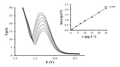
**Figure 4.** DPASV voltammograms of As(V) and its calibration plot (top-right inset) in 0.01 mol L<sup>-1</sup> HCl pH 2 applying an  $E_d$  of -1.30 V and a  $t_d$  of 120 s using a Ag-NS-SPCNFE.
