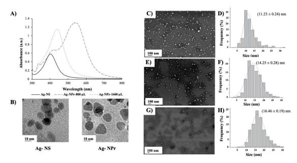
**Figure 1.** (**A**) UV–VIS spectra of Ag-NS, Ag-NPr (800  $\mu$ L), and Ag-NPr (1600  $\mu$ L); (**B**) TEM micrographs for Ag-NS and Ag-NPr (800  $\mu$ L). SEM characterization and corresponding size distribution histograms for the Ag-NS (**C**,**D**) and Ag-NPr obtained using 800  $\mu$ L (**E**,**F**) and 1600  $\mu$ L (**G**,**H**) of Ag-NS as a precursor.
