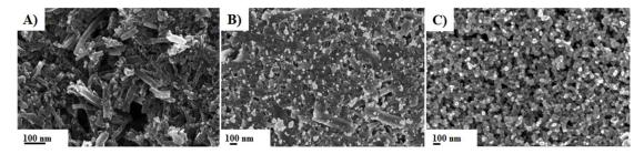
**Figure 2.** SEM micrographs for (**A**) Bare-carbon-nanofiber-based screen-printed electrodes (SPCNFEs) and electrodes modified by drop-casting: (**B**) Ag-NS-SPCNFE and (**C**) Ag-NPr-SPCNFE (800  $\mu$ L).
