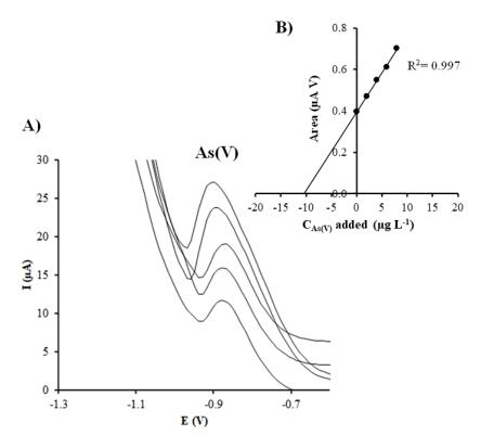
**Figure 5.** (**A**) DPASV measurements of As(V) in a spiked tap water sample on Ag-NS-SPCNFE at pH 2.0 applying an E<sub>d</sub> of -1.30 V and a t<sub>d</sub> of 120 s; and (**B**) As(V) standard addition plot.
